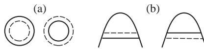
Fig. 1. Schematic structure (a) and energy profile (b) of the double-antidot FQHE qubit. Solid (dashed) lines (in (b), horizontal lines) indicate the edges of the incompressible electron liquid when the quasiparticle is localized at the right (left) antidot. Displacement of the electron liquid is quantized due to quantization of the single-particle states circling the antidots.
