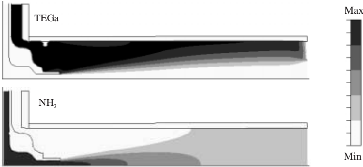
Fig. 1. Concentration profiles of TEGa (upper) and \text{NH}_3 (lower) mass flows inside the reactor chamber for T_D = 800\text{ }^\circ\text{C} , P_{tot} = 200\text{ mbar} and Q_{tot} = 28\text{ slm} from numerical simulations – symmetry axis of the reactor chamber and the inlet are on the left hand side, direction of gas flow is left to right.
