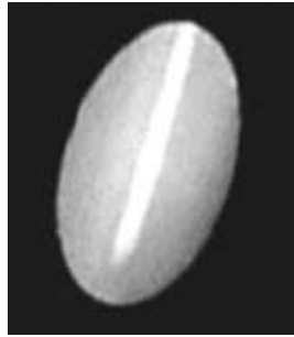
Fig. 2. CL image of the RHEED e-beam track on the structure with 15 CdSe layers and 50 nm thick ZnSe barriers. Oval spot is an area excited by CL e-beam of 5 mm in diameter. The white stripe inside the spot emits in yellow spectral range while the other part of the spot emits in blue-green spectral range.
