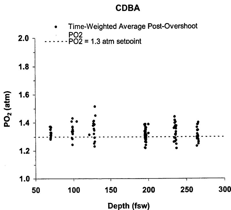
Figure N4. Time weighted average diver inspired PO<sub>2</sub> at bottom after PO<sub>2</sub> overshoots in Royal Navy CDBA. The dotted line is the nominal 1.3 ATA PO<sub>2</sub> set-point of the CDBA.
