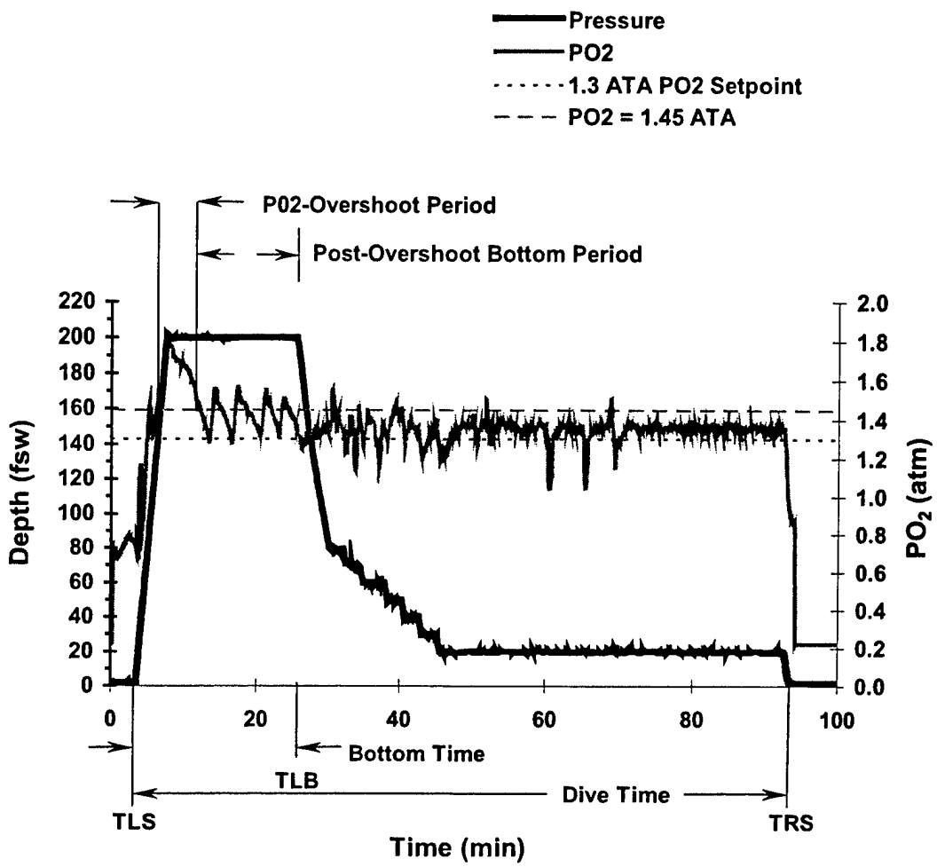
Figure 7. Illustration of different periods in a MK 16 MOD 1 dive used to characterize MK 16 MOD 1 PO<sub>2</sub> control. (First dive in profile 110600BN91.) TLS ≡ Time Leave Surface, TLB ≡ Time Leave Bottom, TRS ≡ Time Reach Surface.
