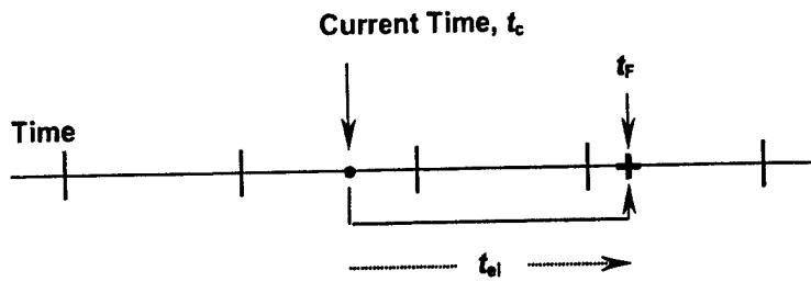
Figure G-7. Generalized instance of the case illustrated in Figure G-6, where mass spectrometer data are not available at  $t_F$ . Latency-corrected interpolated value at  $t_c$  was obtained as schematized in Figure G-8.
