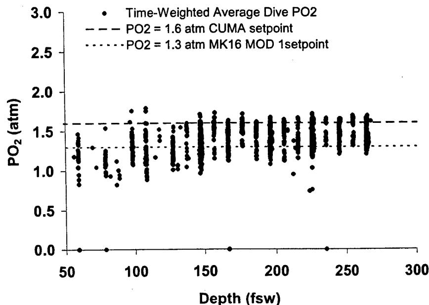
Figure N2. Time weighted average diver inspired PO<sub>2</sub> throughout dive times in CUMA UBA. The heavy dotted line is the nominal 1.6 ATA PO<sub>2</sub> set-point of the CUMA. For comparison, the light dotted line is the nominal 1.3 ATA PO<sub>2</sub> set-point of the MK 16 MOD 1. (Compiled from data provided courtesy of R.Y. Nishi, DCIEM, CA.)
