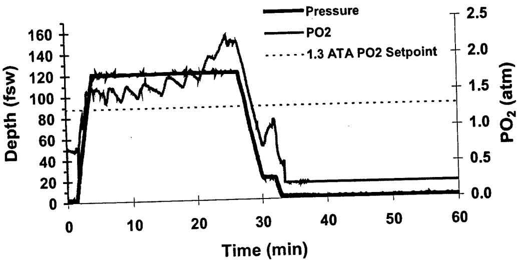
Figure 17. Example of "uncontrolled"  $\text{PO}_2$  increase during bottom phase of first dive in profile 020501BN67. (The complete profile is illustrated in Appendix I. Also see profiles 020801AN67 and 021201AN12 in Appendix I.)
