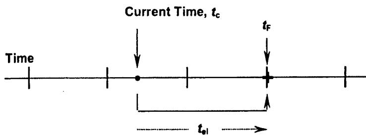
Figure G-5. Schematization of real-time data matrix with mass spectrometer values only at tick marks and fuel cell  $\text{PO}_2$  values at tick marks and at 2 sec intervals in between. In the case illustrated, mass spectrometer data are available at  $t_F$  to obtain latency-corrected interpolated values for the current time,  $t_c$ .
