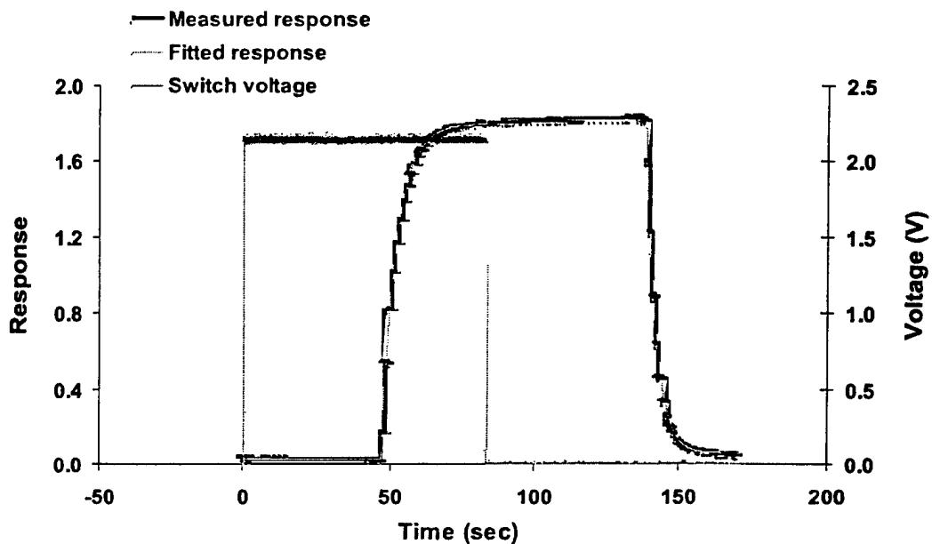
Figure G-2. Typical "ON/OFF" response of mass spectrometer O<sub>2</sub> channel output to near-instantaneous changes in gas concentration at the diver end of the gas sampling umbilical.
