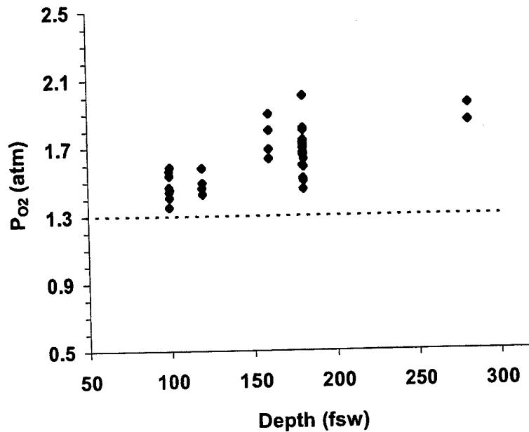
Figure 22. Peak  $\text{PO}_2$  during  $\text{PO}_2$  overshoots in Phase II dives completed using MK 16 MOD 1 UBAs fitted with upgrade R10-DN  $\text{O}_2$  sensors. Dotted line is nominal  $\text{PO}_2$  set-point of the MK 16 MOD 1 UBA at the depths shown.
