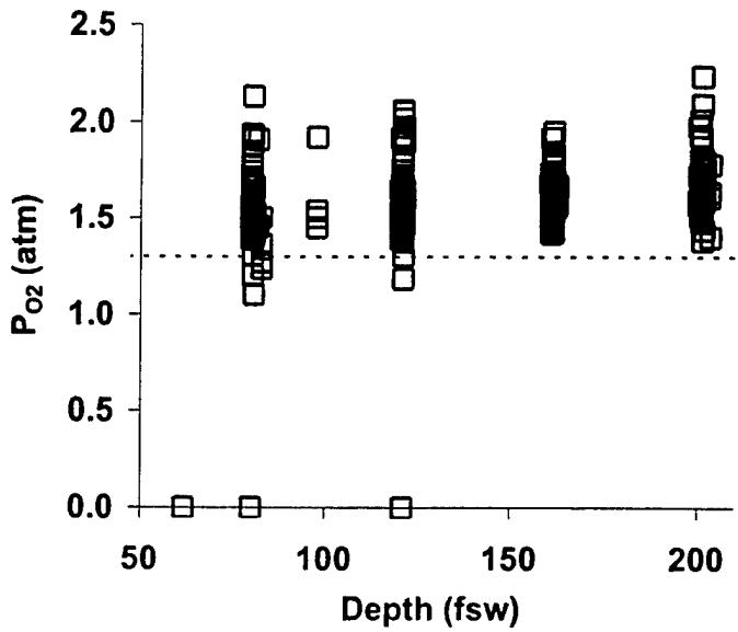
Figure 9. Time-weighted average  $\text{PO}_2$  during  $\text{PO}_2$  overshoot periods in Phase I dives. Dotted line is the nominal 1.3 ATA  $\text{PO}_2$  set-point of the MK 16 MOD 1 at the dive depths shown. Time-weighted Average Overshoot  $\text{PO}_2$  is zero for dives in which no overshoot occurred ( $\text{PO}_2$  did not exceed 1.45 atm during and immediately after descent).
