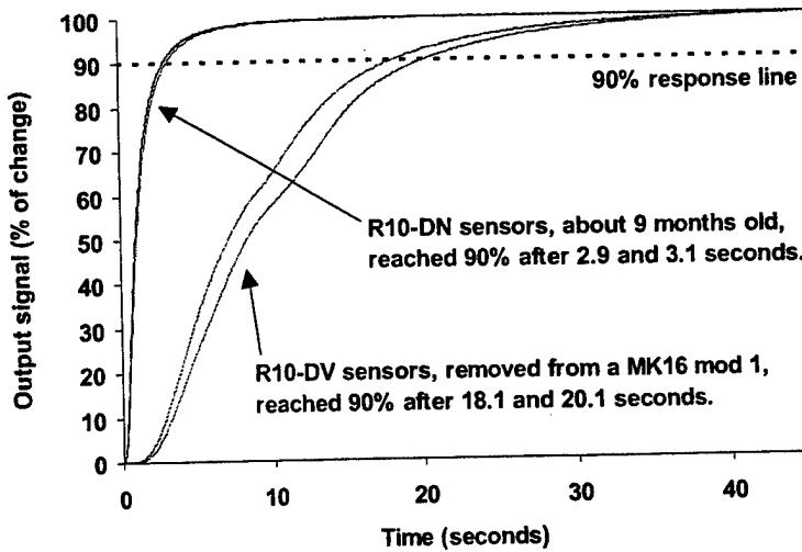
Figure 20. Responses of MK 16 MOD 1  $\text{PO}_2$  sensors to a step change in  $\text{PO}_2$  from 0 to 1 ATA at time = 0. Data for two R10-DV and two upgrade R10-DN sensors are shown.
