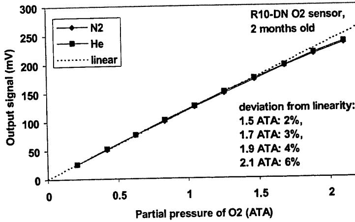
Figure 19. Output vs.  $\text{PO}_2$  of upgrade R10-DN sensors with either  $\text{N}_2$  or He as background gas. The sensors remain linear to within about 5% at  $\text{PO}_2$  up to 2.0 ATA with either background inert gas.
