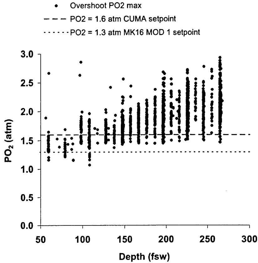
Figure N1. Peak diver inspired  $\text{PO}_2$  in Canadian CUMA UBA. The dotted line is the nominal 1.6 ATA  $\text{PO}_2$  set-point of the CUMA UBA. (Compiled from data provided courtesy of R.Y. Nishi, DCIEM, CA.)
