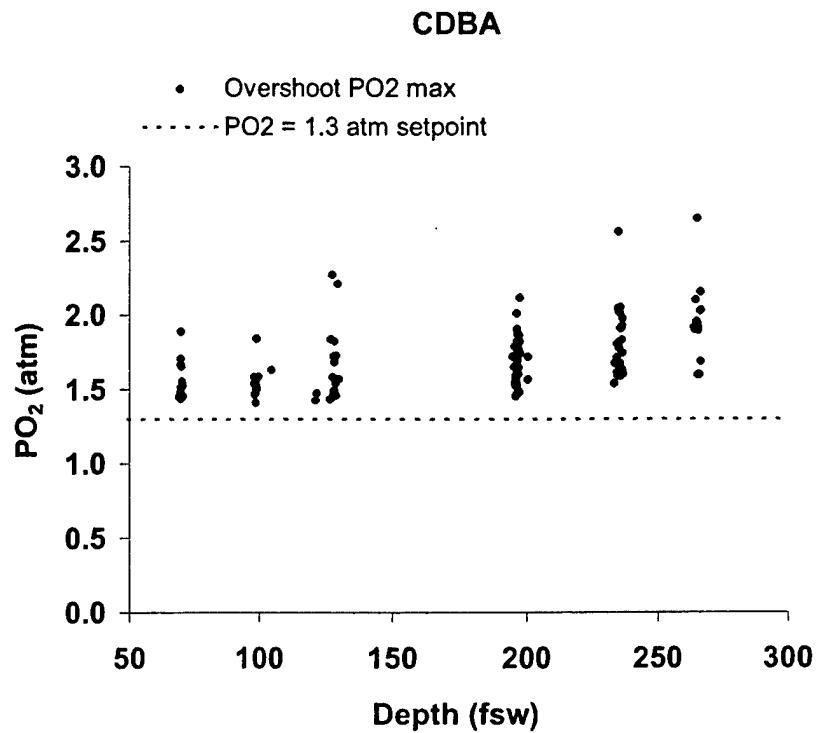
Figure N3. Peak diver inspired PO<sub>2</sub> in Royal Navy CDBA. The dotted line is the nominal 1.3 ATA PO<sub>2</sub> set-point of the CDBA. (Compiled from data provided courtesy of T.G. Anthony, DERA(A), UK.)
