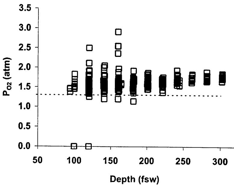
Figure 14. Time-weighted average PO<sub>2</sub> during PO<sub>2</sub> overshoot periods in Phase II dives. Dotted line is the nominal PO<sub>2</sub> set-point of the MK 16 MOD 1 at the dive depths shown. Time-weighted Average Overshoot PO<sub>2</sub> is zero for dives in which no overshoot occurred (PO<sub>2</sub> did not exceed 1.45 atm during and immediately after descent).
