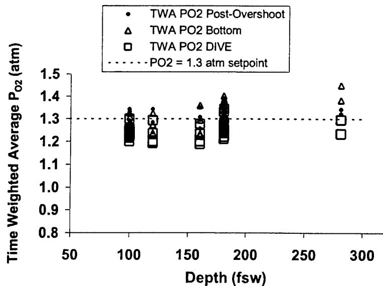
Figure 25. Summary of MK 16 MOD 1  $\text{PO}_2$  control characteristics at bottom after the  $\text{PO}_2$  overshoot periods, during dive bottom times, and throughout the dives, Phase II dives using MK 16 MOD 1 UBAs fitted with upgrade R10 DN oxygen sensors.
