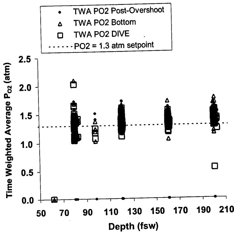
Figure 11. Summary of MK 16 MOD 1  $P_{O_2}$  control characteristics at bottom after the  $P_{O_2}$  overshoot periods, during dive bottom times, and throughout the dives; Phase I dives. Time-weighted Average Post-Overshoot  $P_{O_2}$  is zero for dives in which no overshoot occurred ( $P_{O_2}$  did not exceed 1.45 atm during and immediately after descent).
