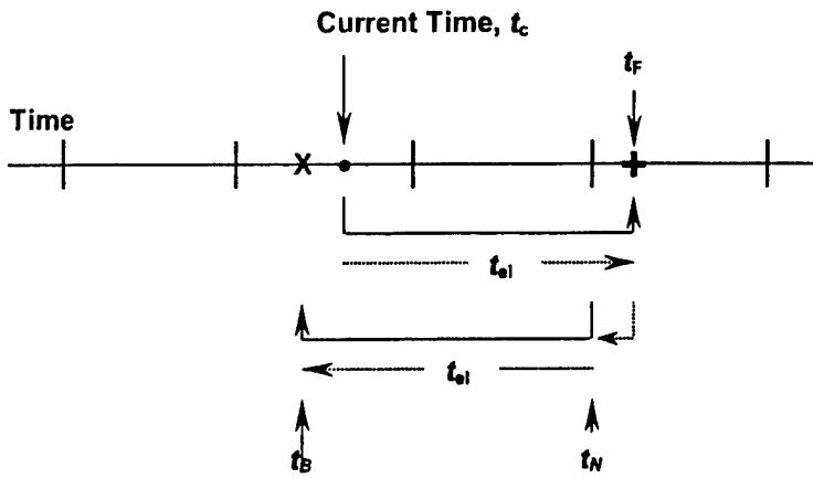
Figure G-8. Determination of the latency-corrected interpolated mass spectrometer data at current time,  $t_c$ , using mass spectrometer data at  $t_N$  and fuel cell data at  $t_B$  when directly measured mass spectrometer data at  $t_f$  were not available.
