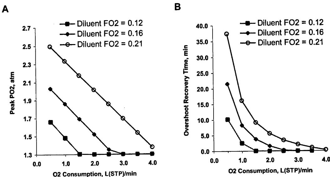
Figure B1. Effects of diluent  $x_{O_2}$  (= diluent FO<sub>2</sub>) on the peak  $P_{O_2}$  (Panel A) and duration of the  $P_{O_2}$  overshoot (Panel B) in a diver with 5 l pulmonary vital capacity compressed on the MK 16 MOD 1 to 300 fsw at 60 fsw/min.
