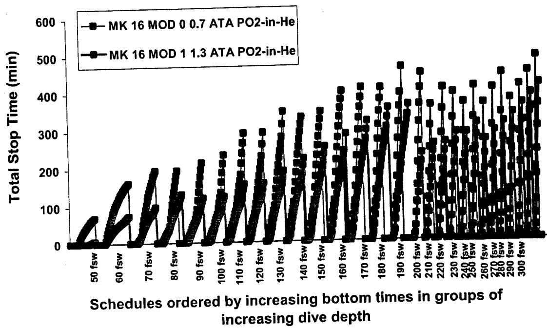
Figure 28. Comparison of total decompression stop times of single dive schedules in the MK 16 MOD 0 Constant 0.7 ATA PO<sub>2</sub>-in-He tables with those of single dive schedules in the new MK 16 MOD 1 1.3 ATA PO<sub>2</sub>-in-He tables.
