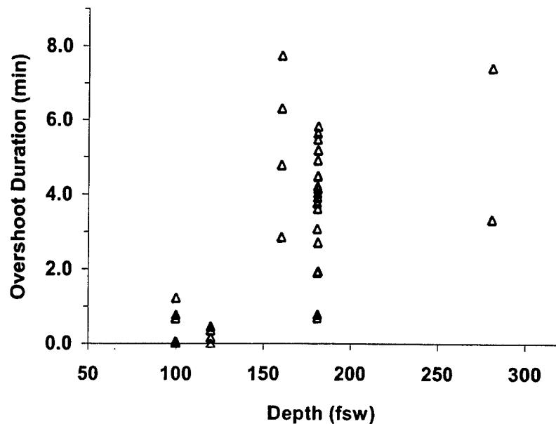
Figure 24. Duration of  $\text{PO}_2$  overshoot periods in Phase II dives completed using MK 16 MOD 1 UBAs fitted with upgrade R10-DN  $\text{O}_2$  sensors.  $\text{PO}_2$  overshoot duration is zero for dives in which no overshoot occurred ( $\text{PO}_2$  did not exceed 1.45 atm during and immediately after descent).
