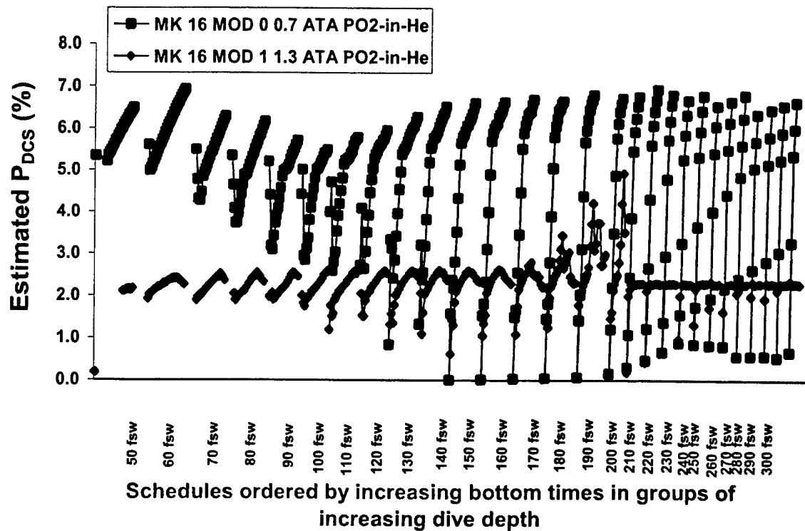
Figure 27. Comparison of estimated DCS risks of single dive schedules in the MK 16 MOD 0 Constant 0.7 ATA PO<sub>2</sub>-in-He tables with those for single dive schedules in the new MK 16 MOD 1 1.3 ATA PO<sub>2</sub>-in-He tables.
