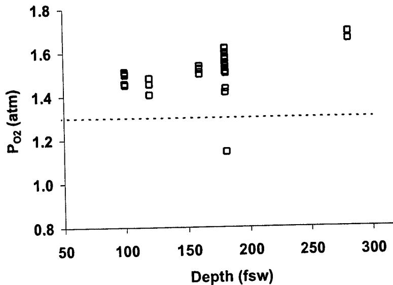
Figure 23. Time-weighted average  $\text{PO}_2$  during  $\text{PO}_2$  overshoot periods in Phase II dives completed using MK 16 MOD 1 UBAs fitted with upgrade R10-DN  $\text{O}_2$  sensors. Dotted line is nominal  $\text{PO}_2$  set-point of the MK 16 MOD 1 UBA at the depths shown.
