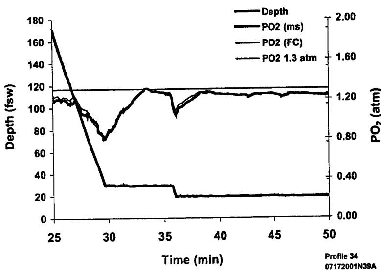
Figure G-9. Section of a profile: A) before fuel cell  $\text{PO}_2$  data smoothing and correction and interpolation of mass spectrometer  $\text{FO}_2$  data, and; B) after fuel cell  $\text{PO}_2$  data smoothing and correction and interpolation of mass spectrometer  $\text{FO}_2$  data.
