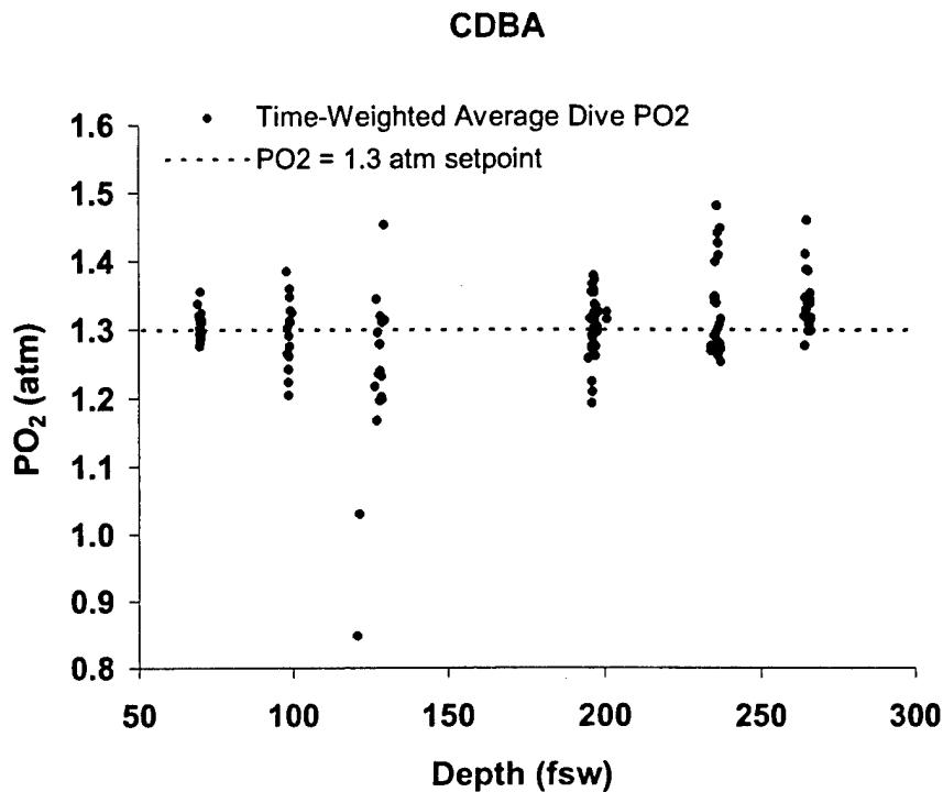
Figure N5. Time weighted average diver inspired PO<sub>2</sub> throughout dive times in Royal Navy CDBA. The dotted line is the nominal 1.3 ATA PO<sub>2</sub> set-point of the CDBA.
