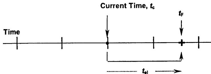
Figure G-6. Schematization of real-time data matrix as in Figure G-5. Here, however, mass spectrometer data are not available at  $t_F$  to obtain latency-corrected values for the current time,  $t_c$ . Note that the mass spectrometer data at  $t_c$  apply to an earlier real time, as illustrated in Figure G-5, and the latency-corrected value at  $t_c$  must be determined by interpolation of the value at  $t_F$ .
