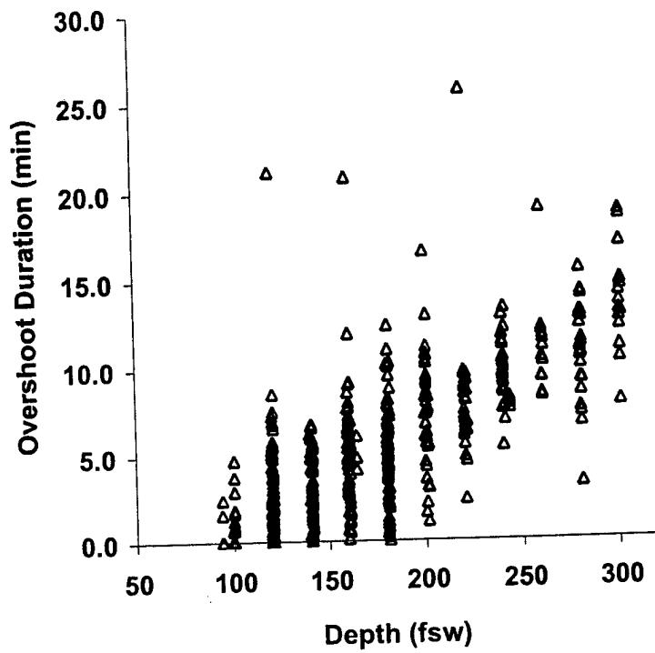
Figure 15. Duration of  $\text{PO}_2$  overshoot periods in Phase II dives.  $\text{PO}_2$  overshoot duration is zero for dives in which no overshoot occurred ( $\text{PO}_2$  did not exceed 1.45 atm during and immediately after descent).
