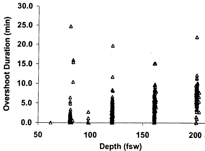
Figure 10. Duration of  $\text{PO}_2$  overshoot periods in Phase I dives.  $\text{PO}_2$  overshoot duration is zero for dives in which no overshoot occurred ( $\text{PO}_2$  did not exceed 1.45 atm during and immediately after descent).
