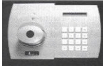
Figure 4.10. Retina Scanner. (From: Nanavati, p. 108).
