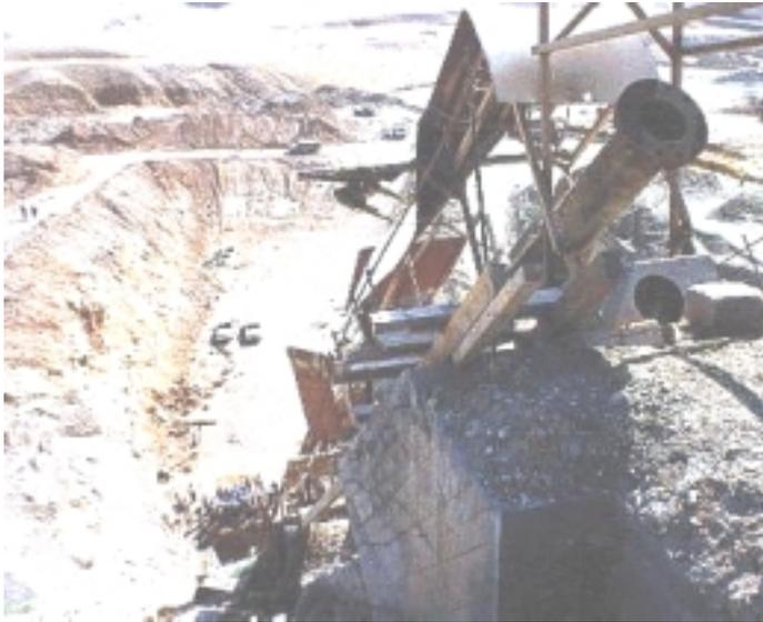
A supergun (termed little Babylon), with 350 mm diameter, as actually built but apparently not tested. This version was built as a fixed direction/launch angle. But it could have been weaponized to a more mobile version.
