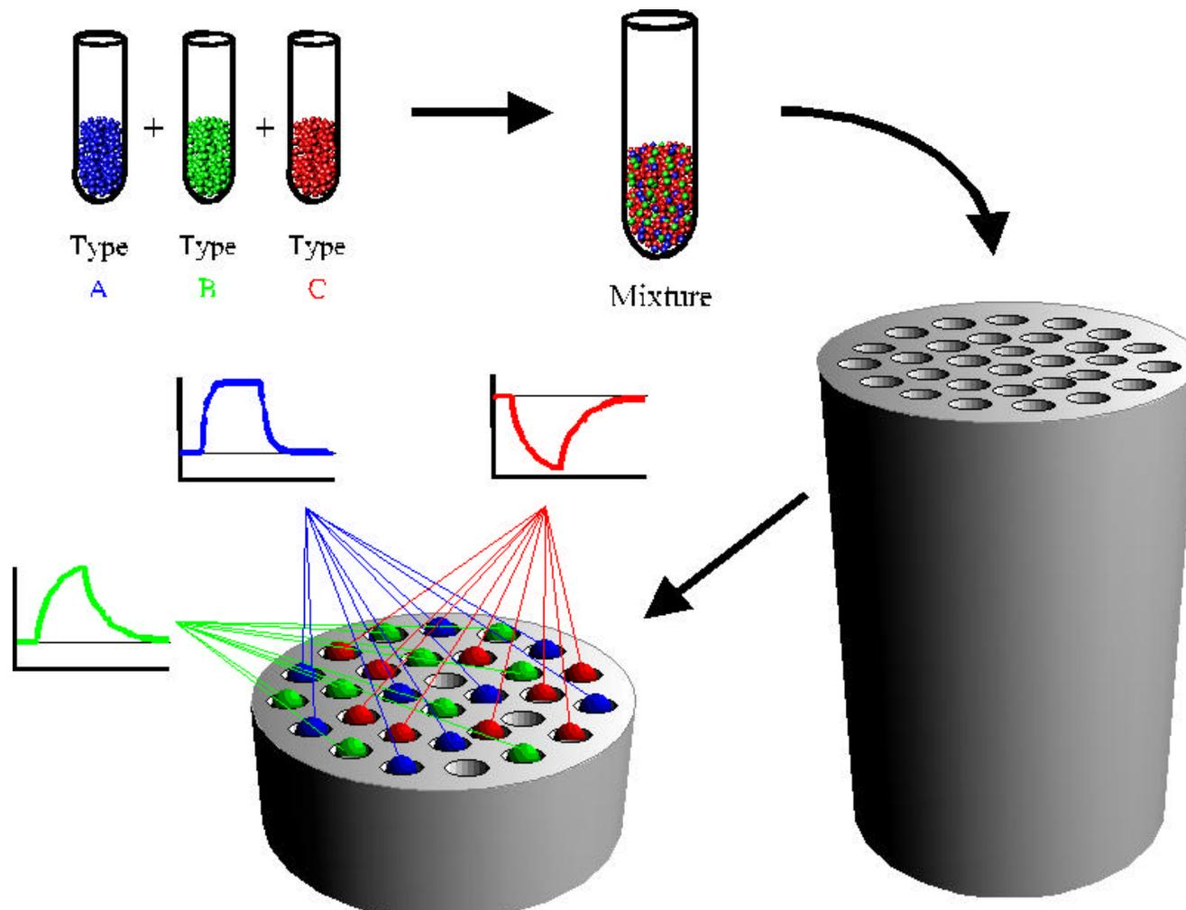
**NOTE: the Sensor Array is a 'Self-Encoding' Bead Array (SEBA). Billions of Sensors are Fabricated at Once.**
