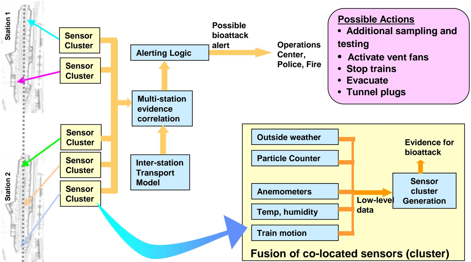
**Multiple sensors required to agree and sensitivity reduced to reduce risk of false alert.**
