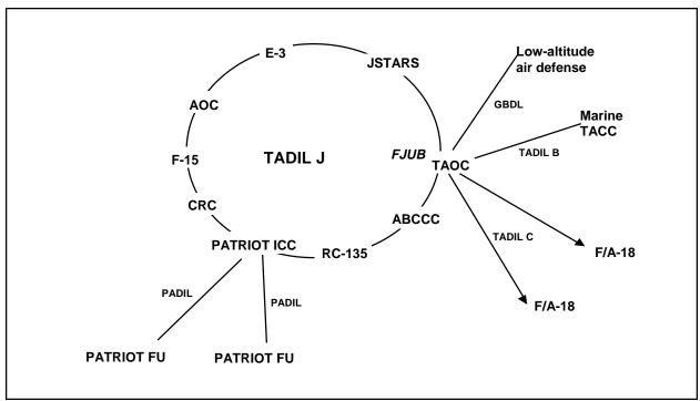
Figure II-3. Joint Architecture Ashore
