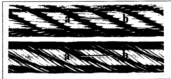
Figure 2-8. The difference in wear characteristics of lang lay and regular lay ropes
