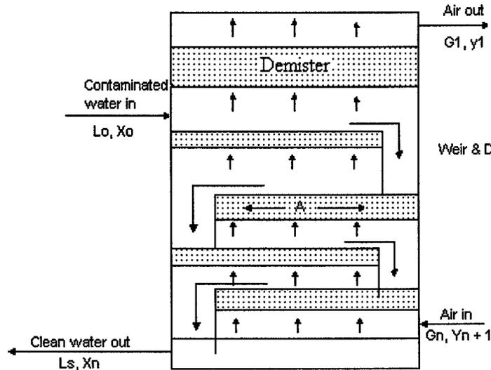
**Figure C-1. Cross-sectional area of perforated plate section.**
