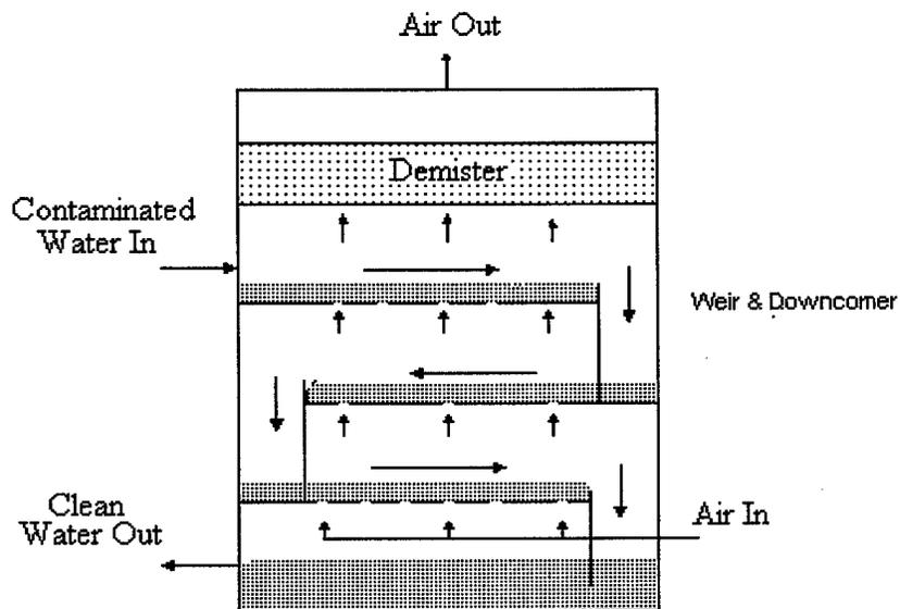
**Figure 2-2. Low profile sieve tray air stripper.**
