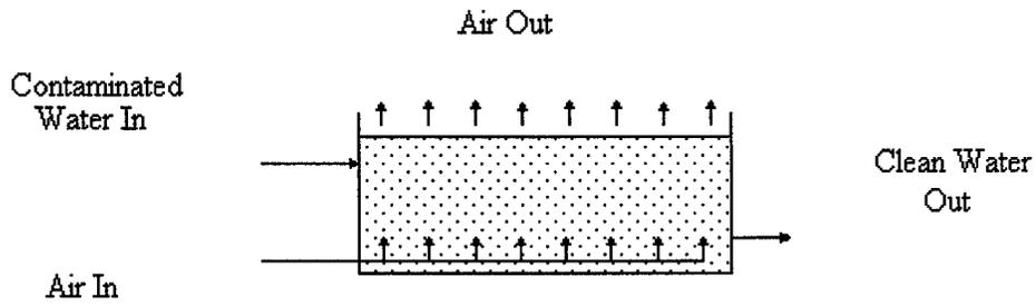
**Figure 2-3. Diffused aeration air stripper.**
