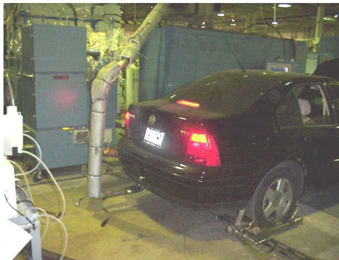
Figure 5. Rear View of Vehicle Test Installation
