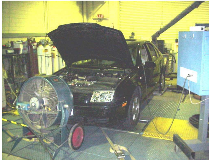
Figure 4. Front View of Vehicle Test Installation
