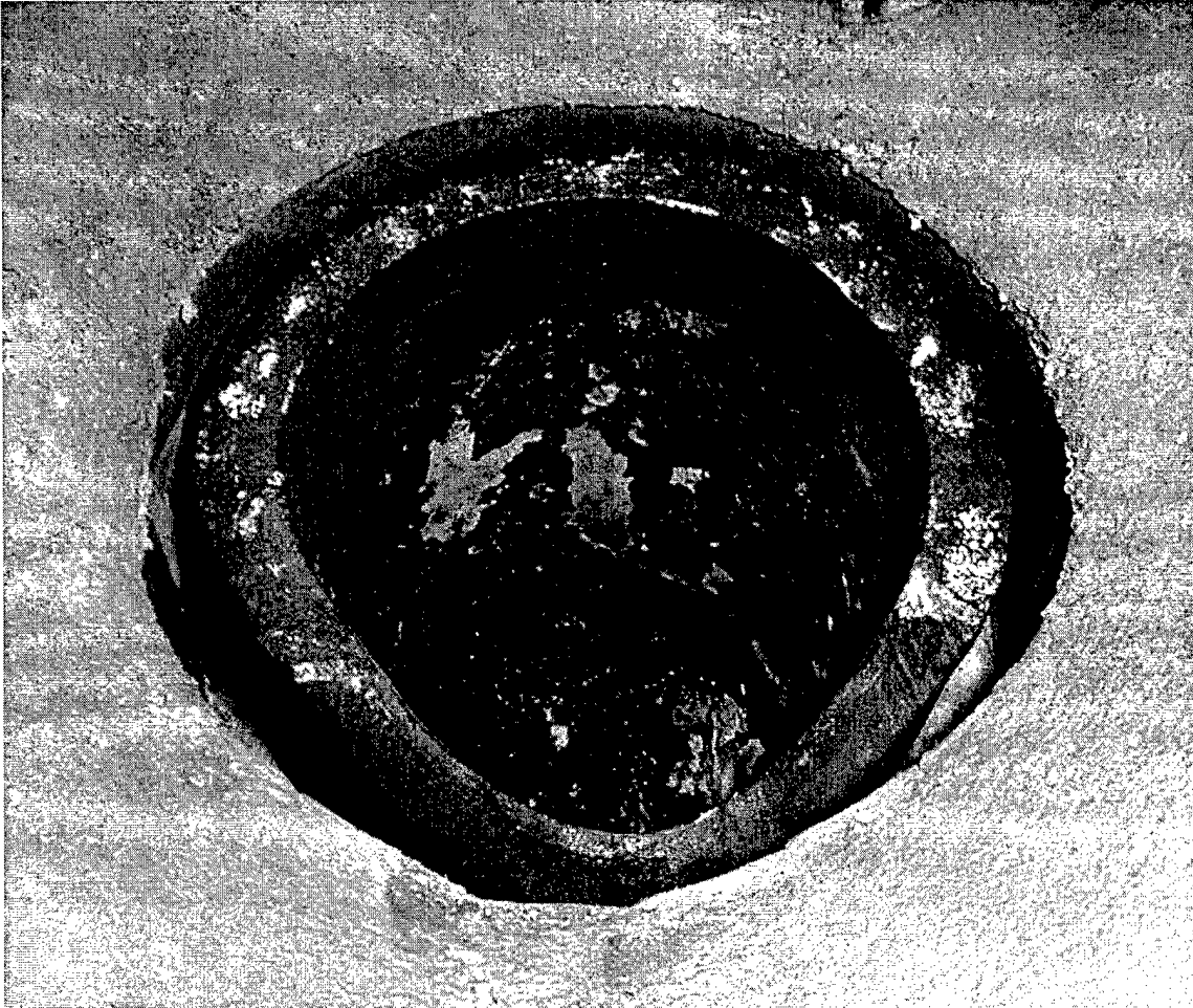
Crucible Modified With Spout & Installed in Refractory
