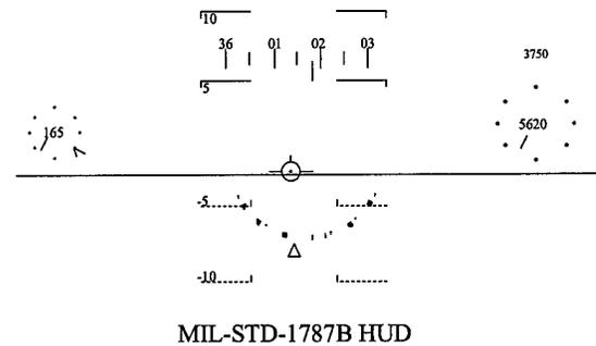
Figure 19. Military standard HUD based on MIL-STD-1787B used as a baseline of comparison for the virtual HUD (see Figure 20). The dial on the left indicates airspeed. The dial on the right indicates altitude. A heading indicator, pitch ladder, bank indicator, flight path indicator and artificial horizon are also included.
