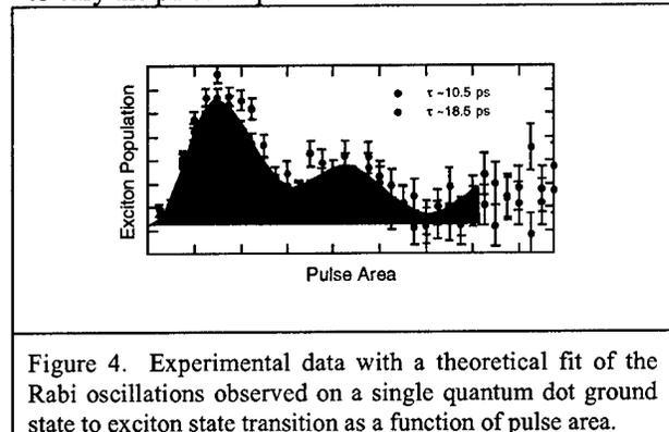
Figure 4. Experimental data with a theoretical fit of the Rabi oscillations observed on a single quantum dot ground state to exciton state transition as a function of pulse area.
