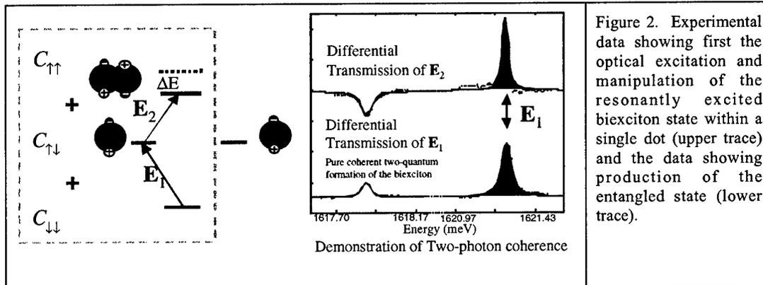
Figure 2. Experimental data showing first the optical excitation and manipulation of the resonantly excited biexciton state within a single dot (upper trace) and the data showing production of the entangled state (lower trace).
