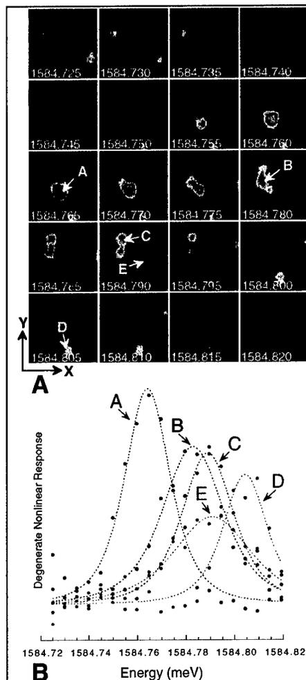
Figure 6. High spectral resolution three-dimensional CW nonlinear response. (A) Three-dimensional CW nonlinear response spanning  $2\mu\text{m} \cdot 2\mu\text{m} \cdot 100\mu\text{eV}$  represented by spatial images recorded at different energies (annotated in  $\text{meV}$ ). (B) The spectral lineshapes for the five eigenstates labeled in (A) are fit by Lorentzians squared
