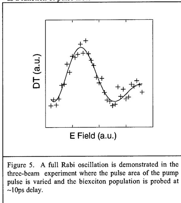
Figure 5. A full Rabi oscillation is demonstrated in the three-beam experiment where the pulse area of the pump pulse is varied and the biexciton population is probed at  $\sim 10$ ps delay.
