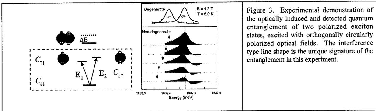
Figure 3. Experimental demonstration of the optically induced and detected quantum entanglement of two polarized exciton states, excited with orthogonally circularly polarized optical fields. The interference type line shape is the unique signature of the entanglement in this experiment.
