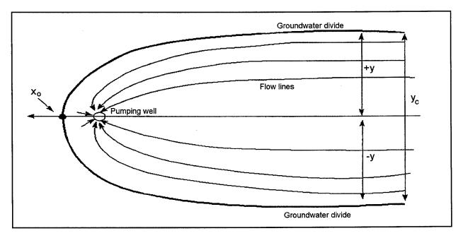
Figure 2-10. Capture zone of a pumping well in plan view. The well is located at the origin (0,0) of the x,y plane
