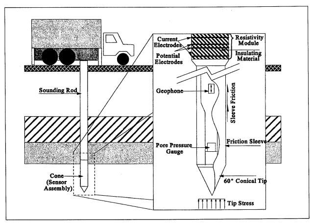
Figure 4-8. Components of cone penetrometer testing system
