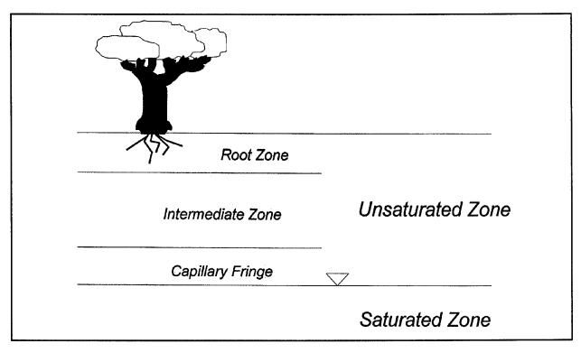
Figure 2-2. Subsurface distribution of water
