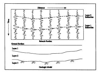
Figure 4-5. Illustration of seismic section for a hypothetical geologic model
