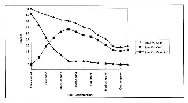
Figure 2-5. Typical relationship between specific yield, specific retention, and total porosity for different soil types
