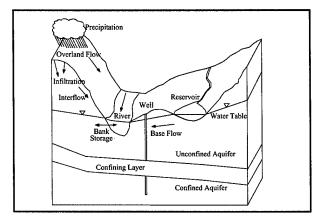
Figure 6-1. Flow components of the surfacegroundwater system
