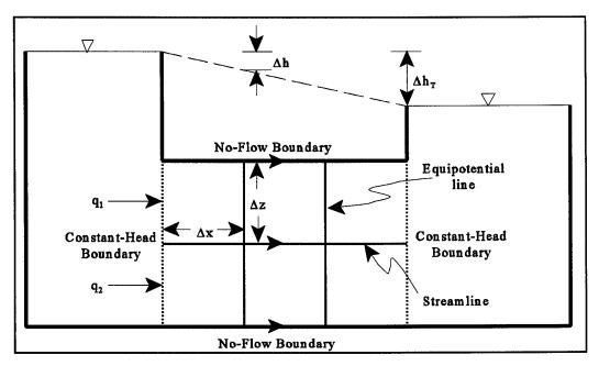
Figure 2-9. Basic flow net
