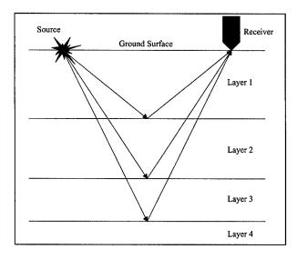
Figure 4-4. Reflected energy from three layers
