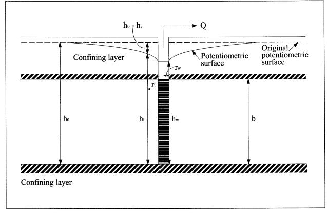
Figure D-1. Parameters used in solution for radial flow to a well in a confined aquifer
