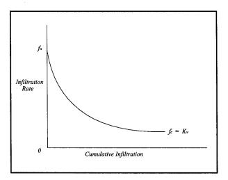
Figure 6-3. Infiltration capacity curve
