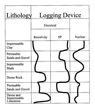
Figure 4-3. Conjunctive use of borehole geophysical logs
