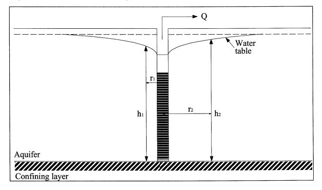
Figure D-2. Parameters used in solution for radial flow to a well in an unconfined aquifer
