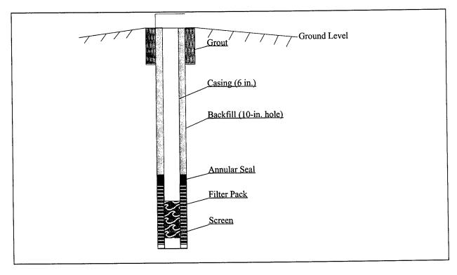
Figure 4-1. Basic well components
