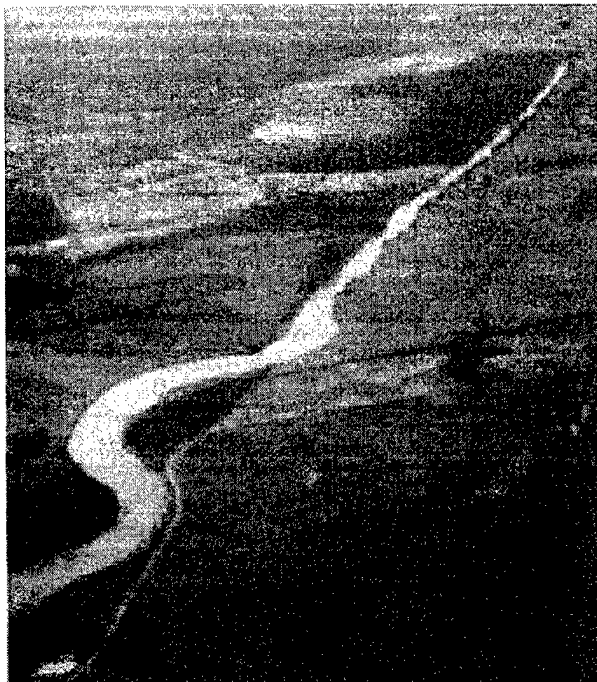
Figure 6-21. Redevelopment of meanders in straightened channel following side bar development
