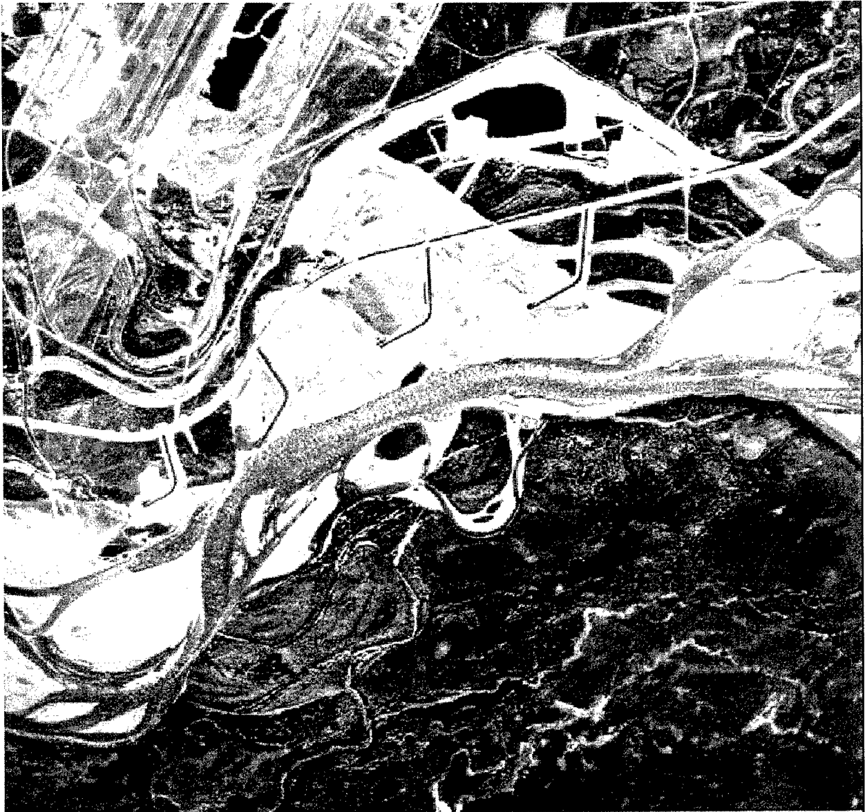
Figure 3-20. Tanana River at Fairbanks showing in-river levee and groins
