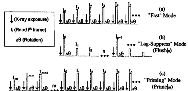
Fig. 4. Timing diagram showing three step-and-shoot acquisition modes. The arrow symbolizes delivery of an x-ray exposure, the \Delta\theta symbol represents an incremental rotation, and the I_i symbol represents readout of the i th frame. For each timing sequence, the pulses drawn in solid lines indicate recorded frames (i.e., projection data that are written to file and used in the CBCT reconstruction), whereas dashed lines indicate frames that are discarded. Furthermore, the height of each pulse is intended to illustrate the pixel signal magnitude (e.g., in the unattenuated beam). The nominal acquisition mode is the "fast" mode (a), in which an exposure is delivered between each image frame. In "lag-suppression" mode (b), n frames are flushed between projections. In "priming" mode, the system is brought closer to signal equilibrium before the actual scan by means of m exposures, rotations, and readouts carried out prior to the first recorded projection. The hypotheses suggest that reconstructed images from "fast" mode should exhibit both the comet and streak artifacts, those from "lag-suppression" mode should exhibit reduced comet and streak, and those from "priming" mode should exhibit reduced streak.
