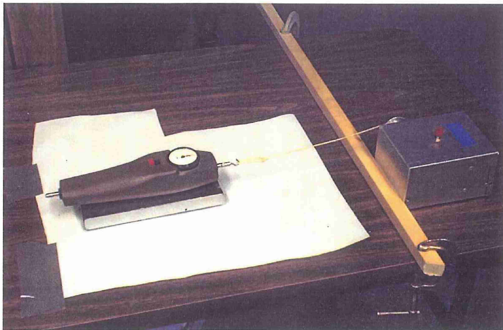
Figure 1. Apparatus and Setup for Measuring Slip Index.
