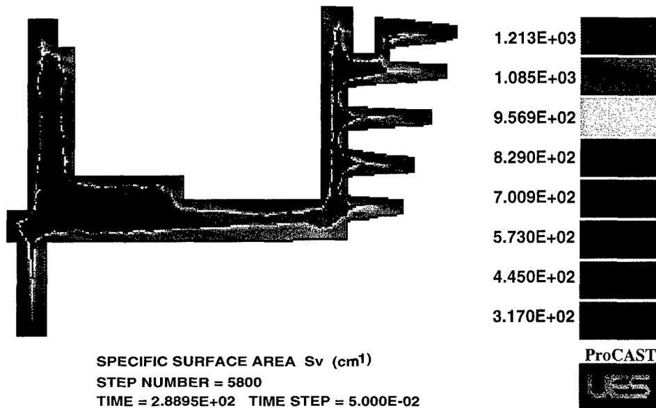
Fig. 5 — Calculated specific surface area  $S_v$  for the as-cast structure of an Al-7%Si brake drum casting based on the mesoscale equiaxed solidification model. (Units of  $S_v$  in the right-hand scale are  $\text{cm}^{-1}$ .)
