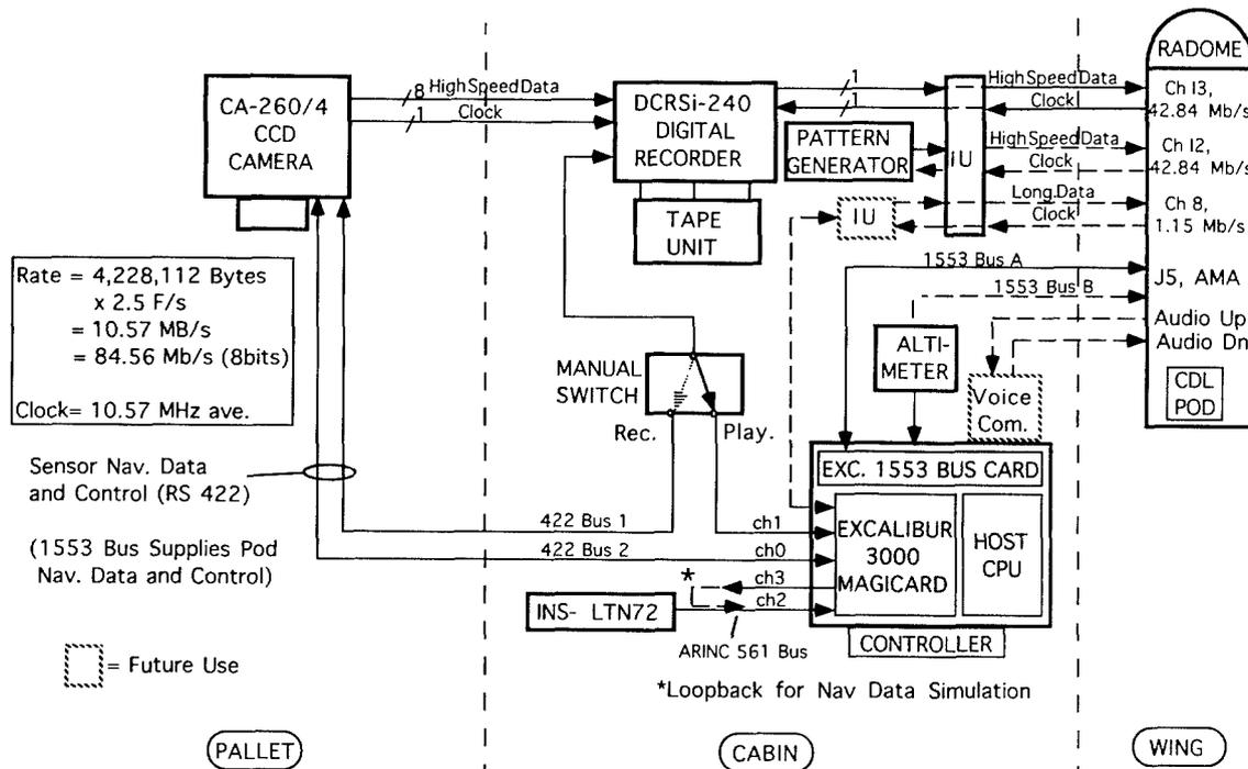
Fig. 2 — Airborne equipment integrated for NRL P-3.
