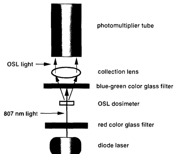
Fig. 4 — An optically stimulated luminescence (OSL) dosimeter system.
