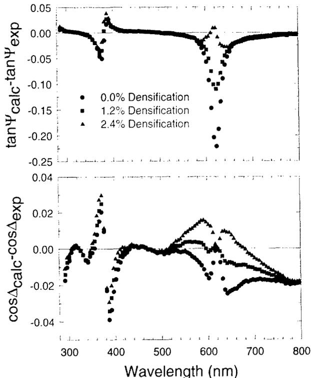
Fig. 20 — Differences between the calculated and experimentally determined values of the spectroscopic ellipsometry parameters  $\tan\Psi$  and  $\cos\Delta$  for an oxide approximately 400-nm thick on a silicon substrate. The calculated values are obtained by assuming that the oxide is densified by either 0.0%, 1.2%, or 2.4%.
