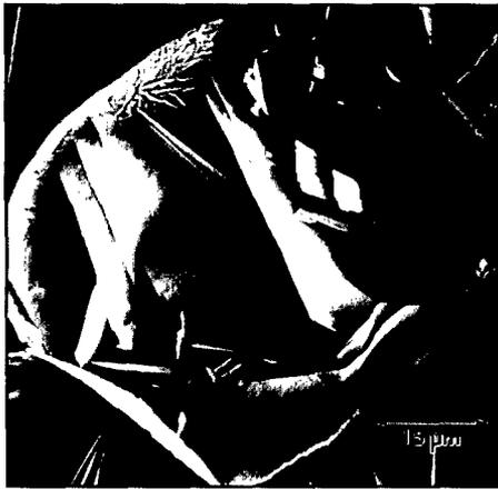
Fig. 8 — Scanning electron micrograph (SEM) of a single austenite grain in a sample that was isothermally transformed at 650° C for 70 s and then deep etched (to remove the austenite matrix), revealing the cementite grain boundary film structure and cementite sideplates and sidelaths.
