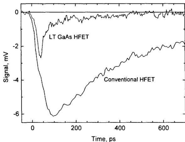
Fig. 2 — 3 MeV  $\alpha$ -particle-induced drain charge-collection transients measured for an  $n$ -channel HFET device with and without the LT GaAs buffer layer (into a 50  $\Omega$  load).  $V_G = 0$  V;  $V_S = 0$  V;  $V_D = 4$  V for the LT device; and  $V_D = 1.5$  V for the conventional device.
