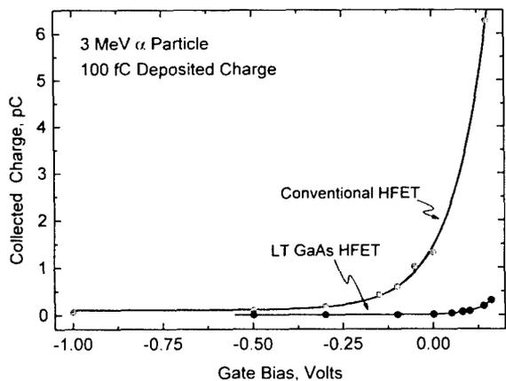
Fig. 3 — Time-integrated charge-collection measurements performed as a function of gate bias for irradiation by 3 MeV  $\alpha$  particles.  $V_D = 2$  V;  $V_S = 0$  V.
