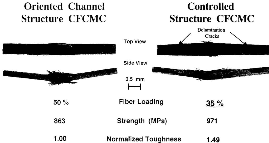
Fig. 3 — Comparison of failure mechanisms and mechanical properties, which illustrates the improvements possible through control of the composite microstructure. These specimens were tested with the matrix channels *parallel* to the applied load similar to the orientation in Fig. 1(b).
