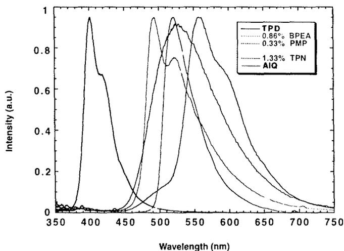
Fig. 9 — Fluorescence spectra of films of TPD, AlQ<sub>3</sub>, and molecular composites of AlQ<sub>3</sub> doped with 9,10-bis(phenylethynyl)anthracene (BPEA), 1,3,5,7,8-pentamethylpyrromethene difluoroborate complex (PMP), quinacridone (DHQ), and 5,6,11,12-tetraphenylnaphthacene (TPN).
