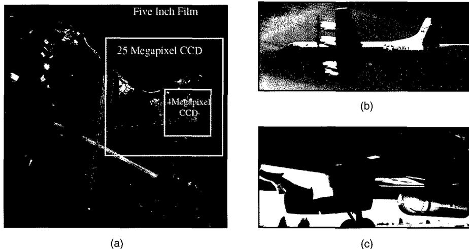
Fig. 1 — (a) Relative areas recorded by KS-87 film camera and CA-260 EO cameras; (b) NRL P-3 flying pallet containing KS-87 film camera and ROI CA-260 CCD camera; and (c) closeup of bolt-on pallet and CDL pod.
