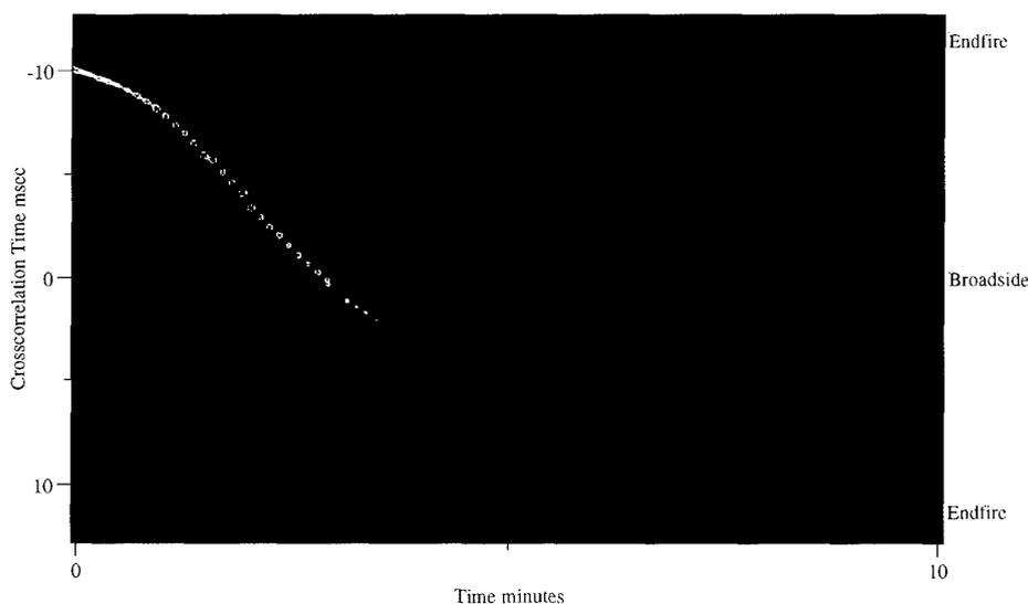
Fig. 4 — Crosscorrelation of a passing vessel.
