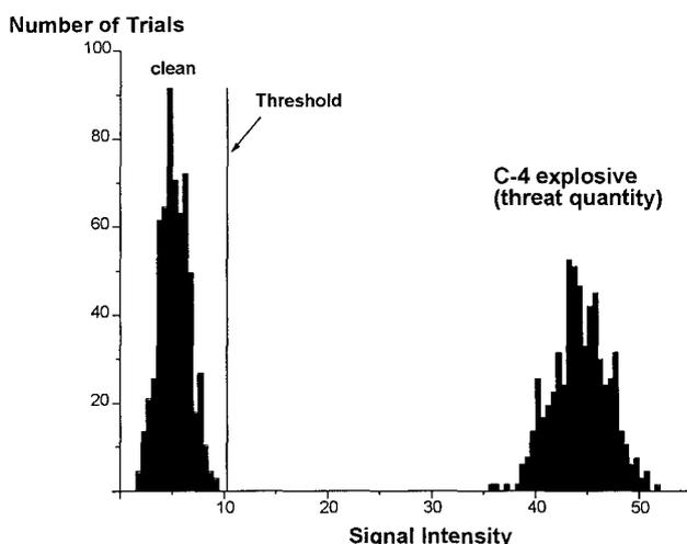
Fig. 8 — Statistical trial histogram showing <sup>14</sup>N NQR signal intensity from a 50-lb piece of luggage, either "clean" or packed with a "threat" quantity of the explosive C-4. The adjustable threshold value for the detector was set to provide a 1% false alarm rate (vertical line). Note the excellent distinction between "safe" (clean) and "alarm" (threat) conditions.
