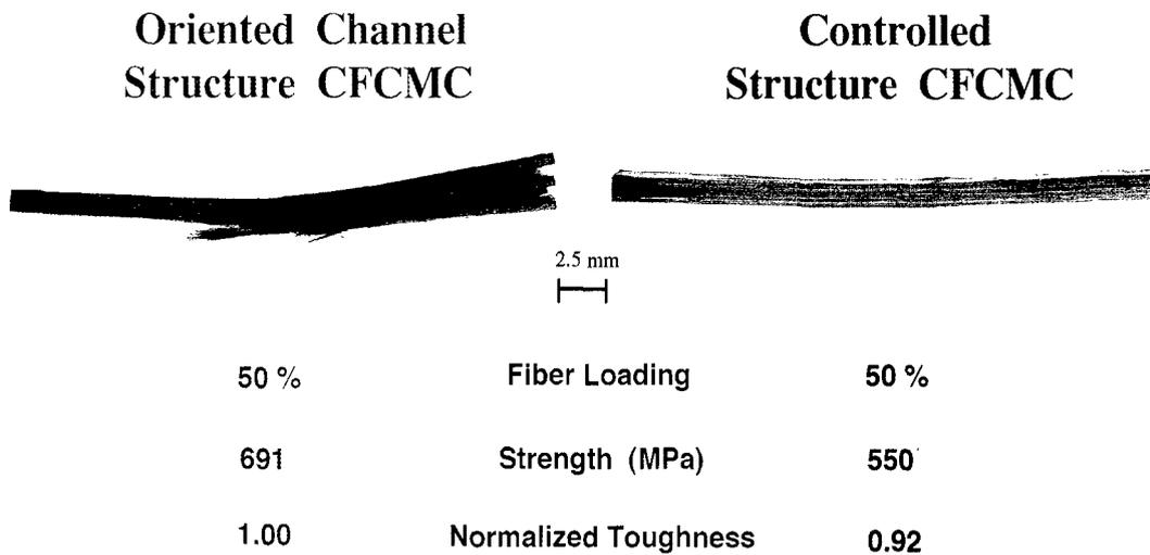
Fig. 4 — Comparison of failure mechanisms and mechanical properties, which illustrates the retention of postfracture structural integrity possible through control of the composite microstructure. These specimens were tested with the matrix channels *perpendicular* to the applied load similar to the orientation in Fig. 1(a).
