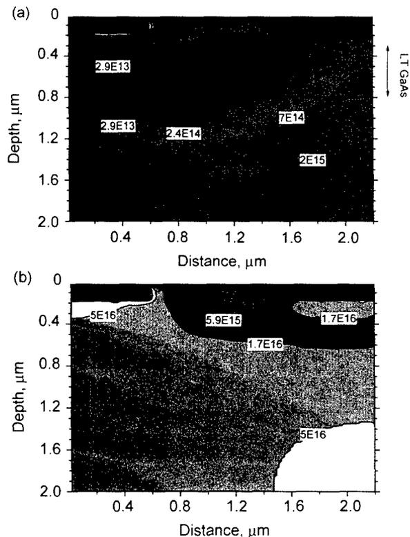
Fig. 4 — Constant electron density contours ( $\text{cm}^{-3}$ ) at 100 ps after the laser pulse for structures (a) with and (b) without a 0.5  $\mu\text{m}$  thick buffer layer with a 1 ps lifetime.  $V_D = 2.5$  V;  $V_G = 0.05$  V; and  $V_S = 0$  V.
