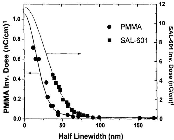
Fig. 6 — Measured linespread widths for SAL-601 and PMMA [4].
