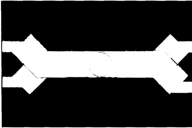
Fig. 5 — Optical micrograph of a typical memory element viewed perpendicular to the film plane. The top metallization is Al, the bottom is Cu and the surrounding blue is  $\text{Si}_3\text{N}_4$ . The stack location is revealed by a circular ring.
