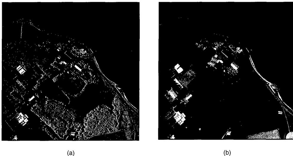
Fig. 3 — Comparison of (a) full size 2K x 2K CA-260 digital electro-optical image and (b) corresponding cropped target region from 5-in. KS-87 film. Visual differences are a result of the extended spectral response of the digital camera and in differences in CCD/film illumination sensitivities.
