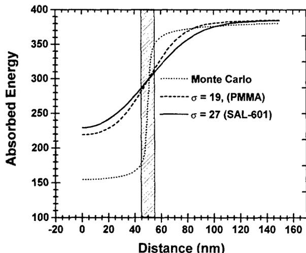
Fig. 7 — Effect of linespread function width on dose latitude for a coded pattern of a 100-nm gap in 20  $\mu\text{m}$  pad. Plotted is the energy absorbed by the resist vs distance from the center of the gap [4].
