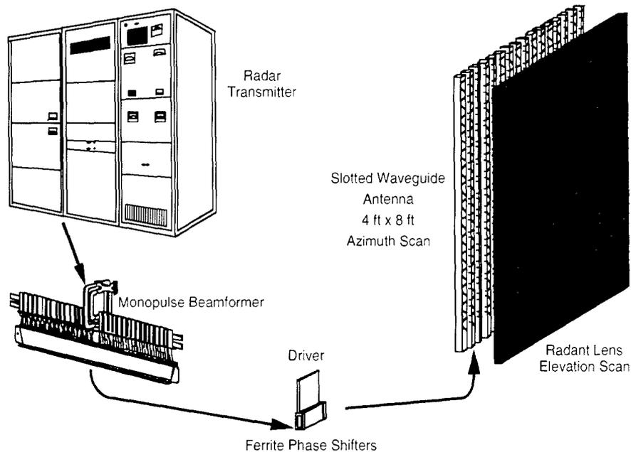
Fig. 2 — Hybrid phased array using Radant lens.
