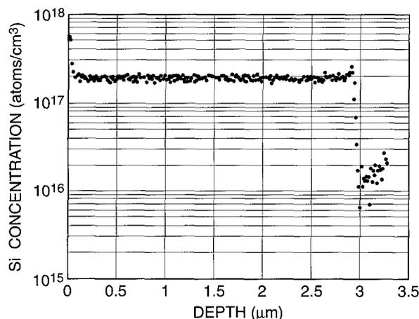
Fig. 17 — SIMS profile of  $^{28}\text{Si}$  atomic concentration as a function of depth for a Si-doped GaN film grown on a highly resistive GaN layer.
