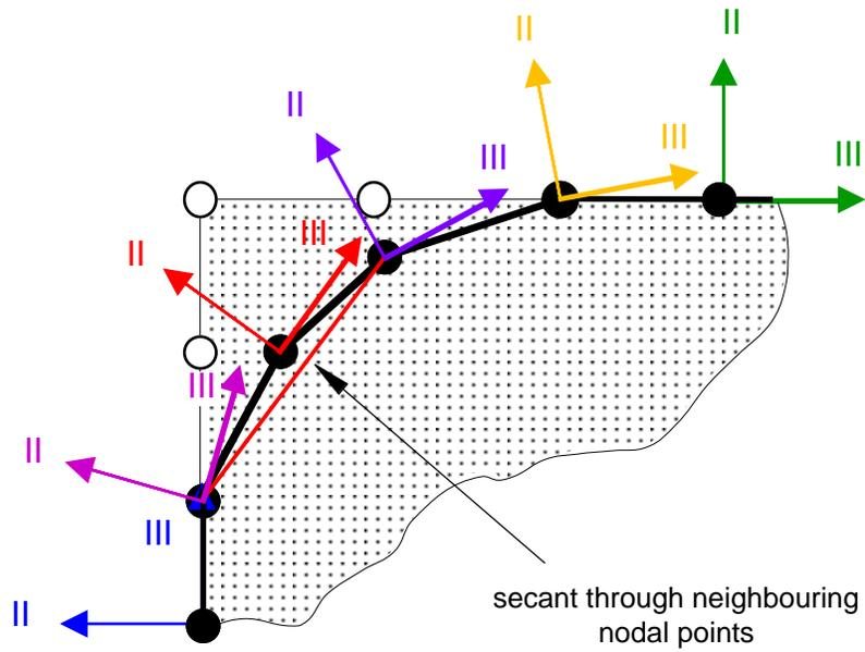
FIGURE 20. Definition of mode separation at sharp corners.
