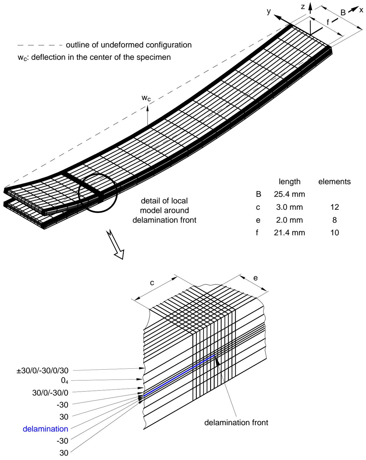
FIGURE 23. Three-dimensional finite element model of SLB specimen.
