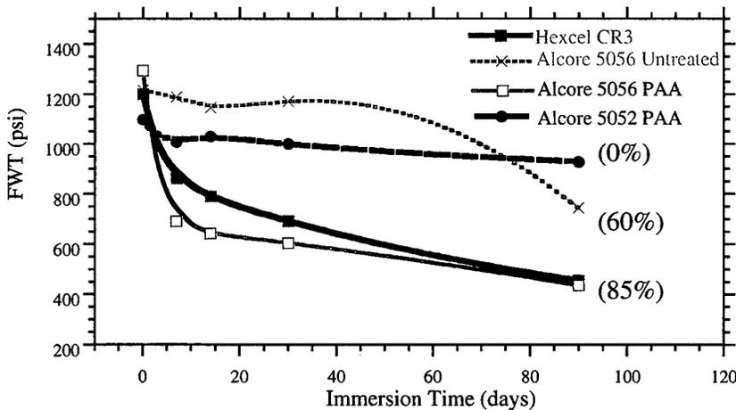
**Figure 4.1.4** FWT strength as a function of immersion time in 95<sup>0</sup>C water for double skinned Alcore and Hexcel honeycomb sandwiches bonded with FM-300.
