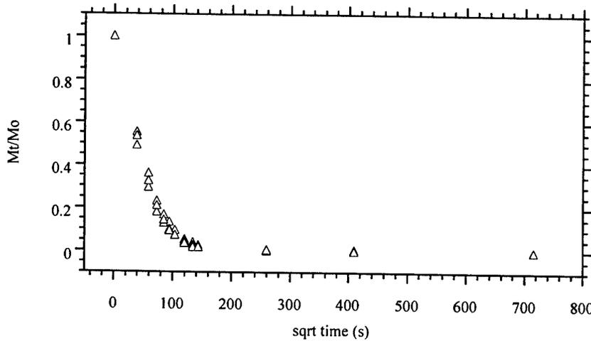
**Figure 4.8.12** Drying rate at in a 80°C isothermal oven for FM-300-2K adhesive saturated by immersion in 70°C water
