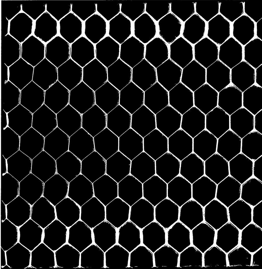
**Figure A3.0** *Hexcel CR3 honeycomb sandwich panel bonded with FM-300 and 0.5mm skins. Image acquired with Kodak M film at 50kV, 12mA/s and normal incidence after 3 days immersion in Cerium Nitrate solution at 70°C.*
