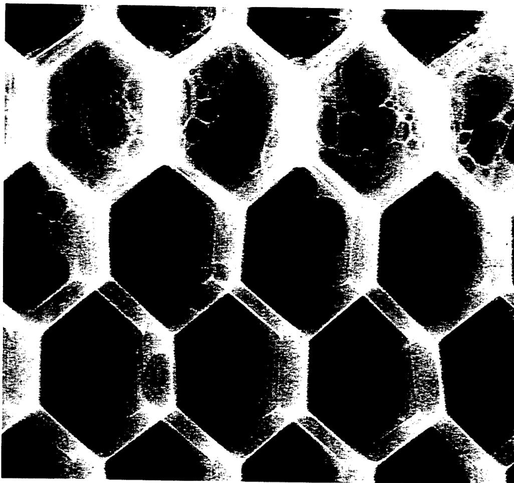
*Figure A2.3 Hexcel CR3 honeycomb sandwich panel bonded with FM-300 and 0.5mm skins. Image acquired with Kodak M film at 50kV, 12mA/s at 5 degrees off normal incidenc after 2 days immersion in Cerium Nitrate solution.*
