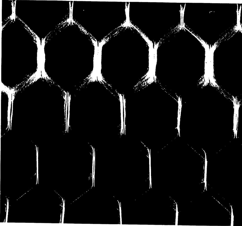
*Figure A3.3 Hexcel CR3 honeycomb sandwich panel bonded with FM-300 and 0.5mm skins. Image acquired with Kodak M film at 50kV, 12mA/s and 5 degrees off normal incidence after 3 days immersion in Cerium Nitrate solution at 70°C.*
