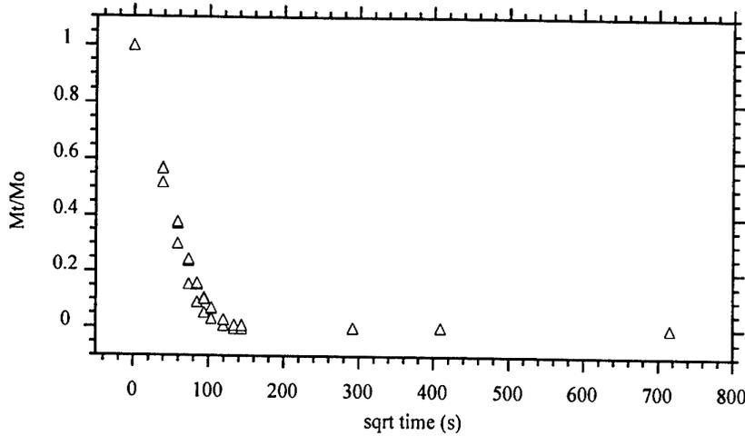
**Figure 4.8.11** Drying rate in a 80°C isothermal oven for FM-300-2K adhesive saturated by immersion in 95°C water
