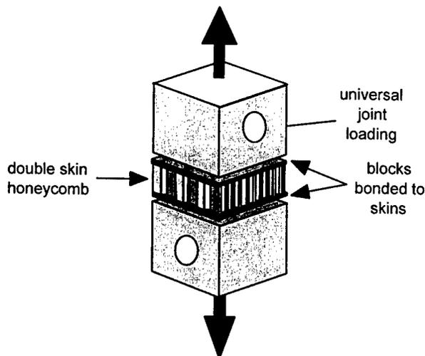
**Figure 2.1** Experimental arrangement for Flat-wise tension testing of Honeycomb sandwiches.
