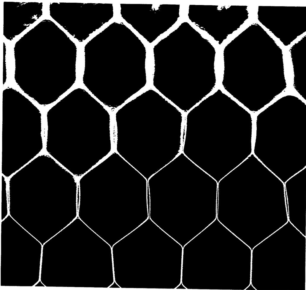
*Figure A5.1 Hexcel CR3 honeycomb sandwich panel bonded with FM-300 and 0.5mm skins. Image acquired with Kodak M film at 50kV, 12mA/s and normal incidence after 10 days immersion in Cerium Nitrate solution at 70°C.*
