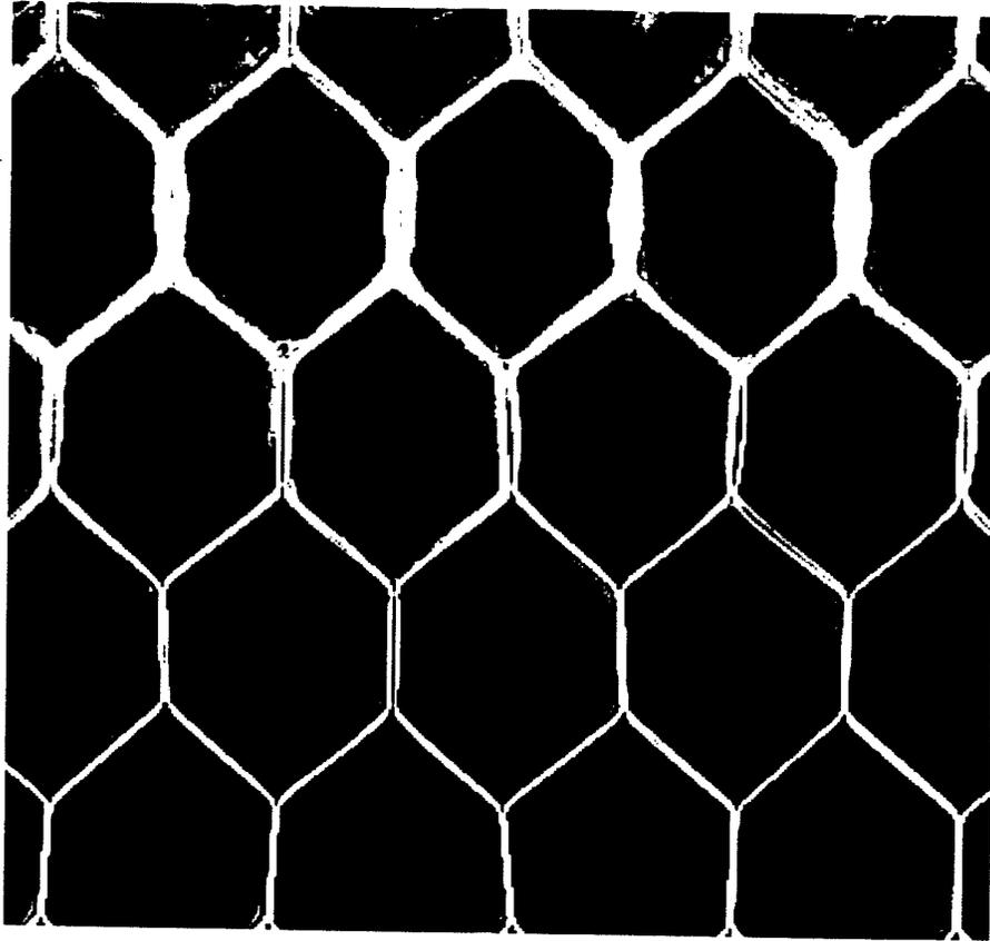
**Figure A4.1** *Hexcel CR3 honeycomb sandwich panel bonded with FM-300 and 0.5mm skins. Image acquired with Kodak M film at 50kV, 12mA/s and normal incidence after 5 days immersion in Cerium Nitrate solution at 70°C.*
