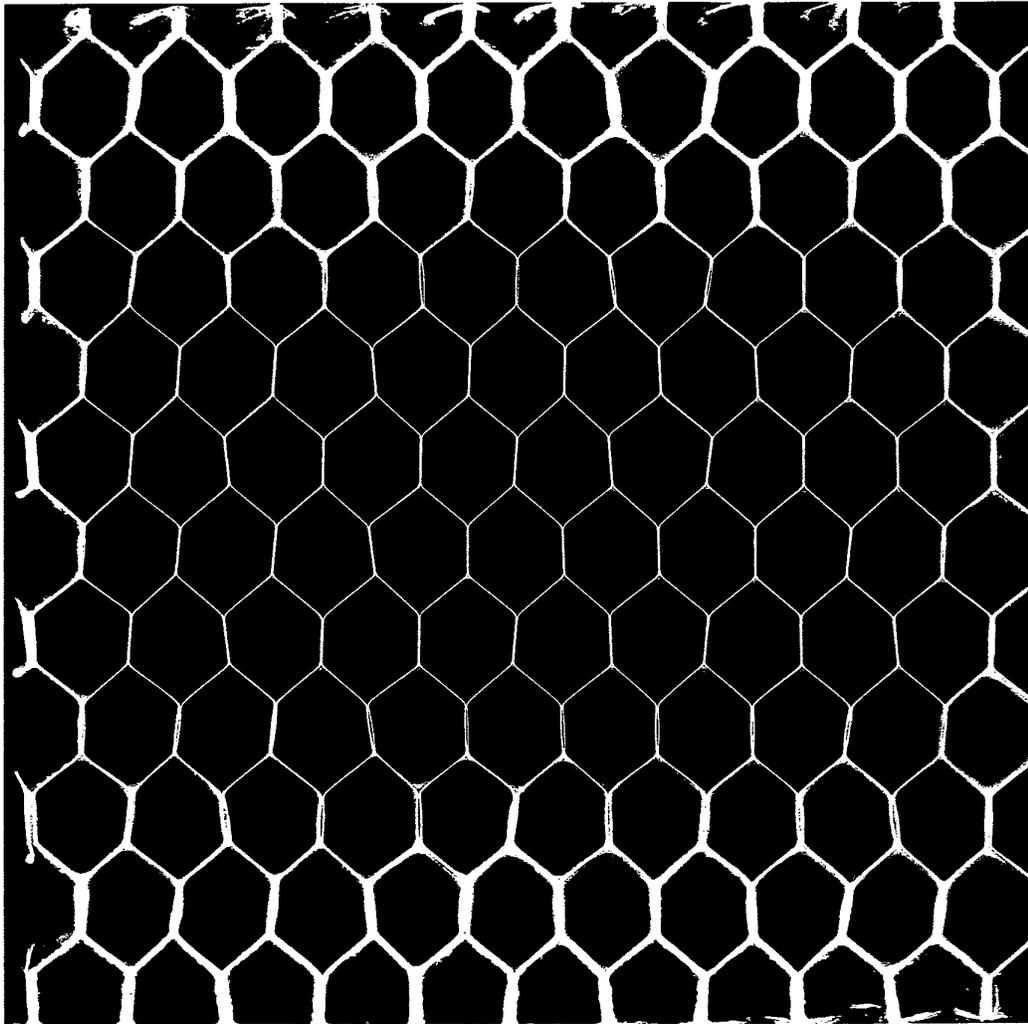
**Figure A5.0** *Hexcel CR3 honeycomb sandwich panel bonded with FM-300 and 0.5mm skins. Image acquired with Kodak M film at 50kV, 12mA/s and normal incidence after 10 days immersion in Cerium Nitrate solution at 70°C.*
