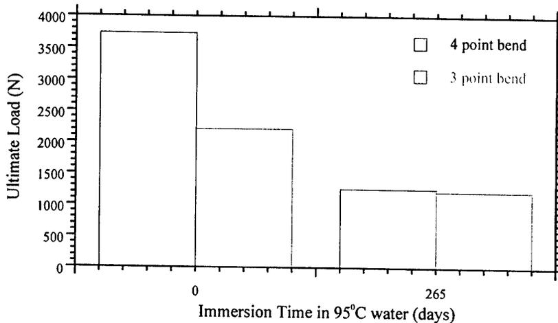
Figure 4.5.4 Ultimate load in 3 and 4 point bending modes for beam samples immersed 9<sup>1</sup>/<sub>2</sub> months in 95°C water, relative to control samples.
