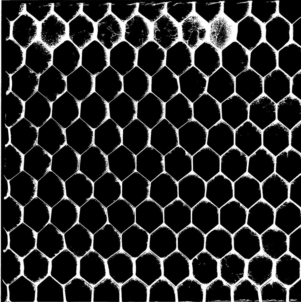
*Figure A2.0 Hexcel CR3 honeycomb sandwich panel bonded with FM-300 and 0.5mm skins. Image acquired with Kodak M film at 50kV, 12mA/s at normal incidence after 2 days immersion in Cerium Nitrate solution.*
