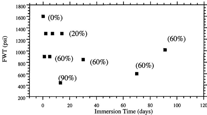
**Figure 4.1.3** FWT strength as a function of immersion time in 95<sup>0</sup>C water for Hexcel CR3 honeycomb. Sandwich sample was immersed in water with only one skin bonded.
