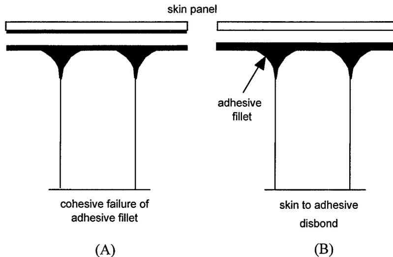
**Figure 2.6** Common failure modes observed for metal honeycomb sandwich construction.
