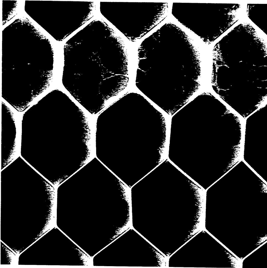
*Figure A2.1 Hexcel CR3 honeycomb sandwich panel bonded with FM-300 and 0.5mm skins. Image acquired with Kodak M film at 50kV, 12mA/s at normal incidence after 2 days immersion in Cerium Nitrate solution.*
