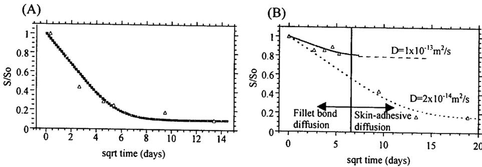
**Figure 5.3.9** *Data fit using equation 5.5 for Hexcel CR3 bonded to(A) FM-300 and (B) FM-300-2K, exposed to 70°C condensing humidity.*
