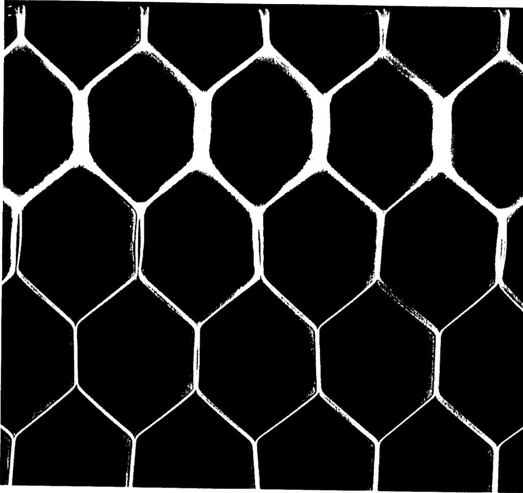
*Figure A3.1 Hexcel CR3 honeycomb sandwich panel bonded with FM-300 and 0.5mm skins. Image acquired with Kodak M film at 50kV, 12mA/s and normal incidence. after 3 days immersion in Cerium Nitrate solution at 70°C.*
