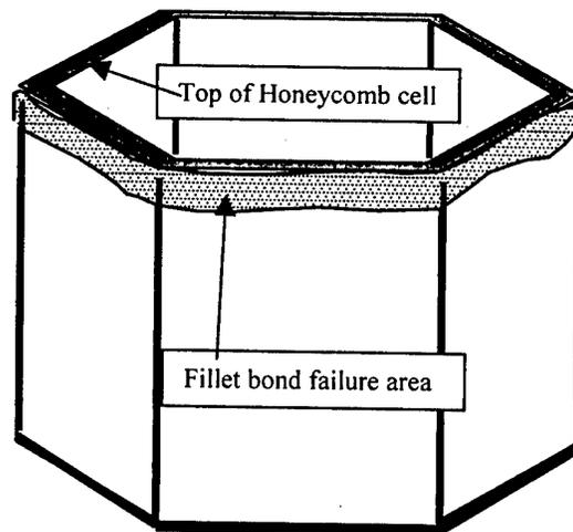
**Figure 4.4.2** The two regions of honeycomb examined using surface analysis
