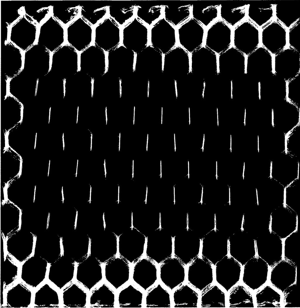
*Figure A5.2 Hexcel CR3 honeycomb sandwich panel bonded with FM-300 and 0.5mm skins. Image acquired with Kodak M film at 50kV, 12mA/s and 5 degrees off normal incidence after 10 days immersion in Cerium Nitrate solution at 70°C.*
