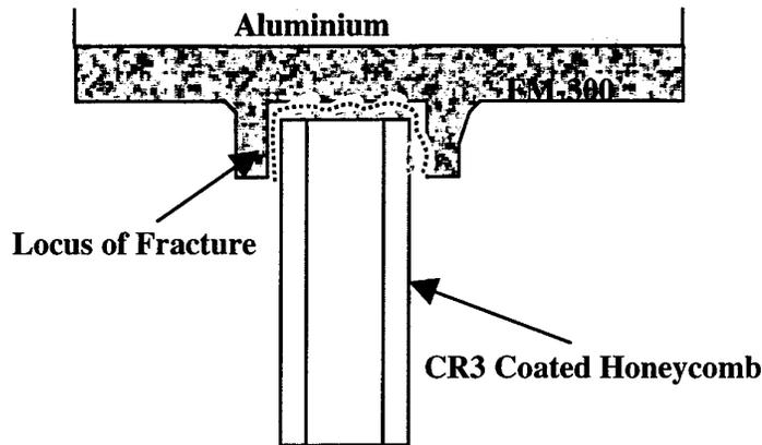
**Figure 4.4.4** Cross-sectional representation of the Hexcel CR3 honeycomb bonded to aluminium with FM-300. The dominant locus of fracture for the FWT sample in the adhesive failure zones tested after 75 days immersion in 95°C water is proposed.
