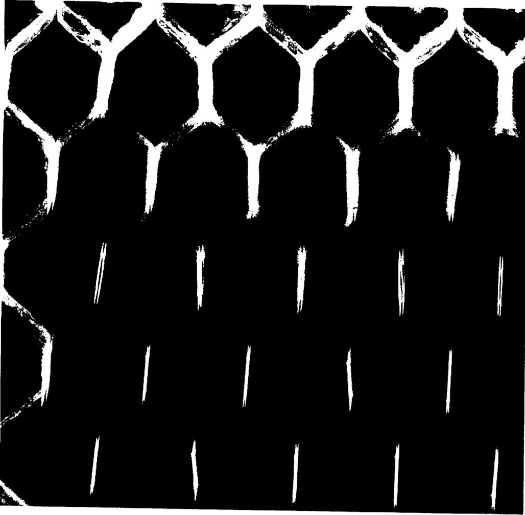
*Figure A5.3 Hexcel CR3 honeycomb sandwich panel bonded with FM-300 and 0.5mm skins. Image acquired with Kodak M film at 50kV, 12mA/s and 5 degrees off normal incidence after 10 days immersion in Cerium Nitrate solution at 70°C.*
