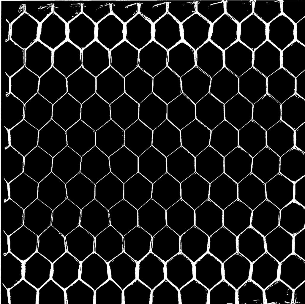
**Figure A4.0** *Hexcel CR3 honeycomb sandwich panel bonded with FM-300 and 0.5mm skins. Image acquired with Kodak M film at 50kV, 12mA/s and normal incidence after 5 days immersion in Cerium Nitrate solution at 70°C.*
