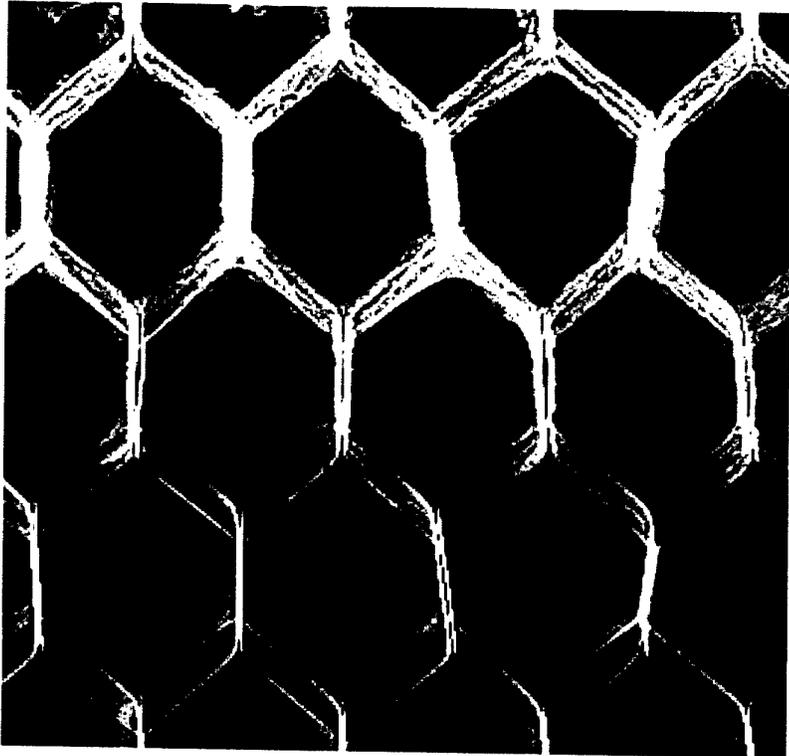
*Figure A4.3 Hexcel CR3 honeycomb sandwich panel bonded with FM-300 and 0.5mm skins. Image acquired with Kodak M film at 50kV, 12mA/s and 5 degrees off normal incidence after 5 days immersion in Cerium Nitrate solution at 70°C.*
