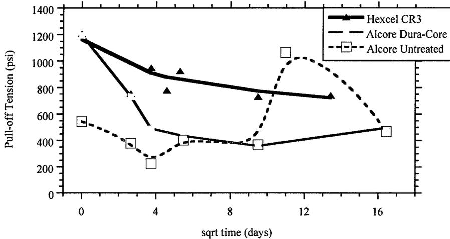
**Figure 4.2.5** Hexcel and Alcore honeycomb bonded to FM-300-2K adhesive and immersed in 70°C water. Pull-off tension as a function of immersion time is indicated.
