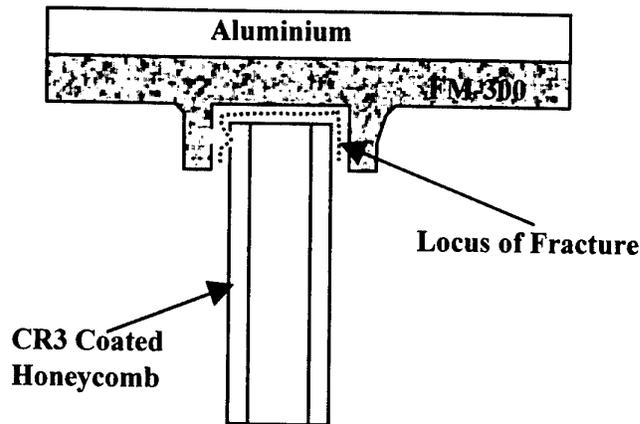
*Figure 4.4.12* Cross-sectional representation of the Hexcel CR3 honeycomb bonded to aluminium with FM-300. The dominant locus of fracture for the Elcometer sample tested after 6 months immersion in 70°C water is proposed.
