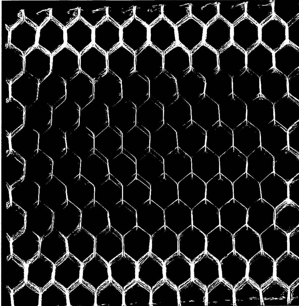
*Figure A4.2 Hexcel CR3 honeycomb sandwich panel bonded with FM-300 and 0.5mm skins. Image acquired with Kodak M film at 50kV, 12mA/s and 5 degrees off normal incidence after 5 days immersion in Cerium Nitrate solution at 70°C.*
