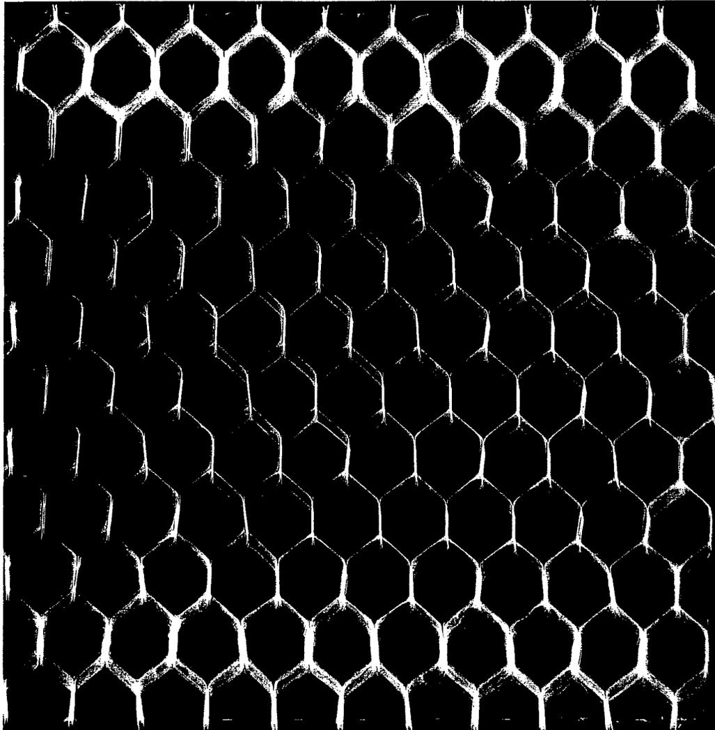
*Figure A3.2 Hexcel CR3 honeycomb sandwich panel bonded with FM-300 and 0.5mm skins. Image acquired with Kodak M film at 50kV, 12mA/s and 5 degrees off normal incidence after 3 days immersion in Cerium Nitrate solution at 70°C.*
