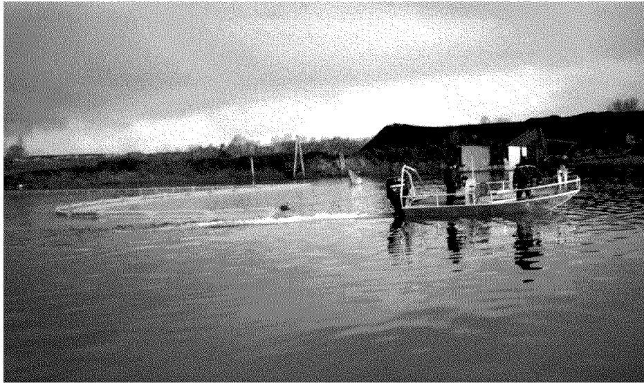
Figure 8-12. A 12-inch draft boom is too much for this boat and motor.
