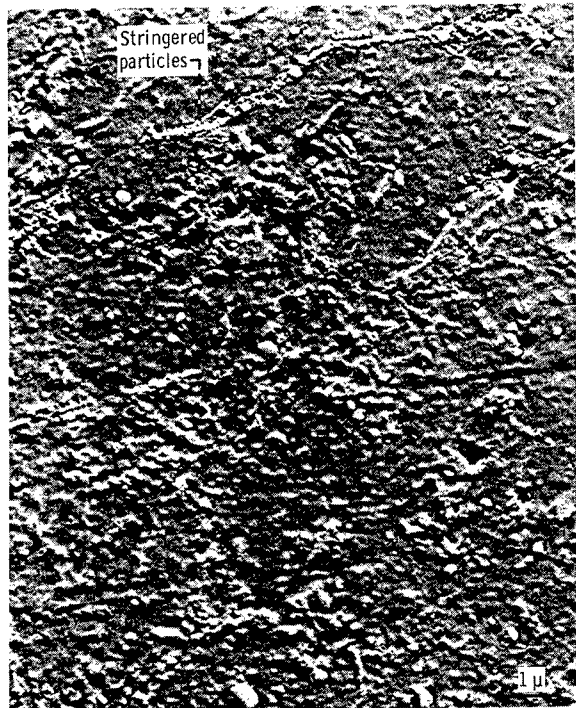
Figure 12. - Blend 4 (nickel - 9.4 volume percent alumina) sintered and compacted with cartridge-actuated compaction press using encapsulation technique.
