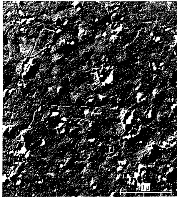
(b) Annealed 4 hours at 1700° F.
