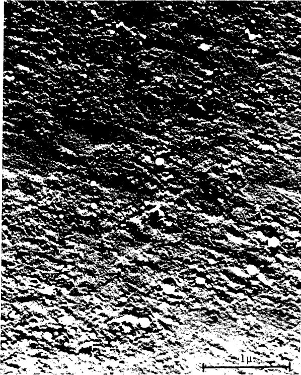
Figure 8. - Blend 1 (nickel - 5 volume percent alumina) hydrogen cleaned at 950° F and compacted in cartridge-actuated compaction press using standard method. Original magnification, X29 250.
