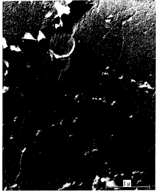
Figure 9. - Blend 2 (nickel - 7.5 volume percent thoria) liquid blended, vacuum dried at 950° F, compacted with cartridge-actuated compaction press using overlay method, and then annealed 1 hour at 1700° F. Original magnification, X29 250.
