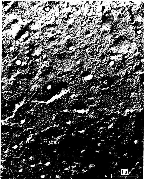
Figure 14. - Blend 5 (nickel - 6.5 volume percent alumina) hydrogen cleaned at 850° F and compacted with Dynapak. Original magnification, X19 000.
