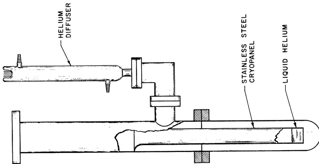
Fig. 7 - System Used on Adsorption Isotherm Experiment. The Cryopanel (Liquid Helium Filled Finger) and Diffuser Shown in the Drawing Form the Left Column of the Vacuum System Shown in the Photograph.
