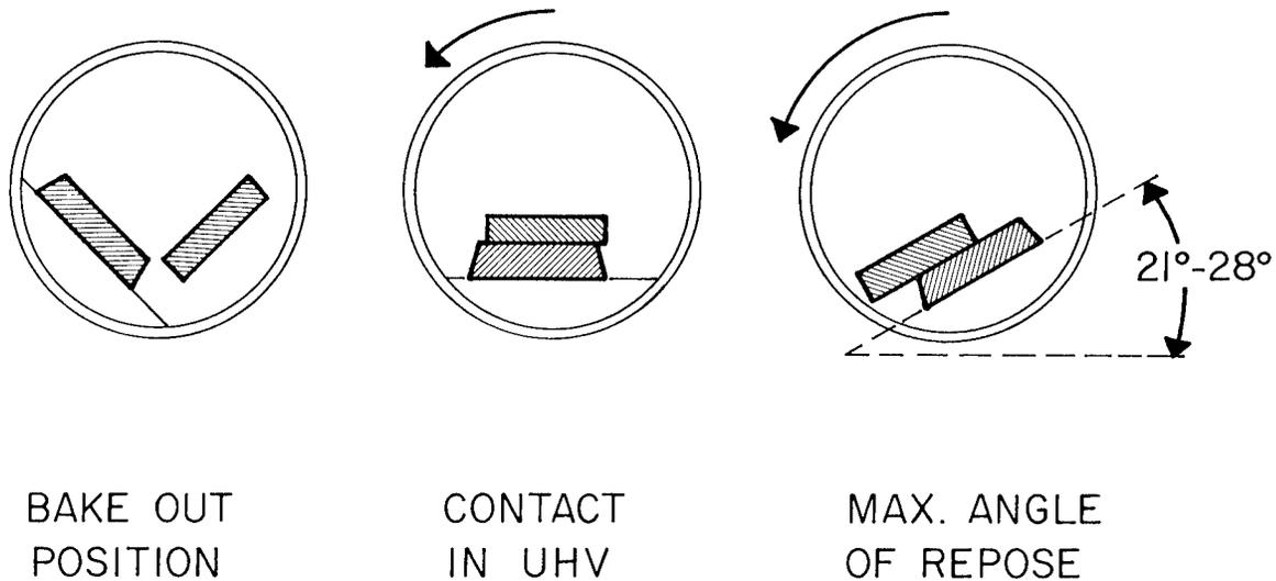
Fig. 8 - Illustration of a Technique for Alternately Exposing the Surfaces of Two Samples to Vacuum Degassing and Bringing the Same Surfaces Into Contact for an Adhesion Measurement
