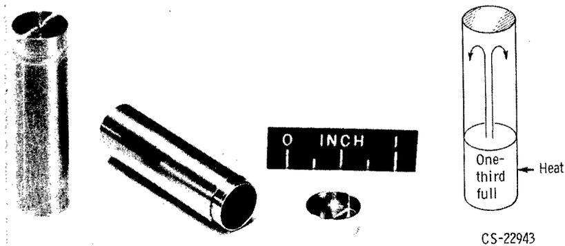
Figure 1. - Reflux capsule used in potassium corrosion study.
