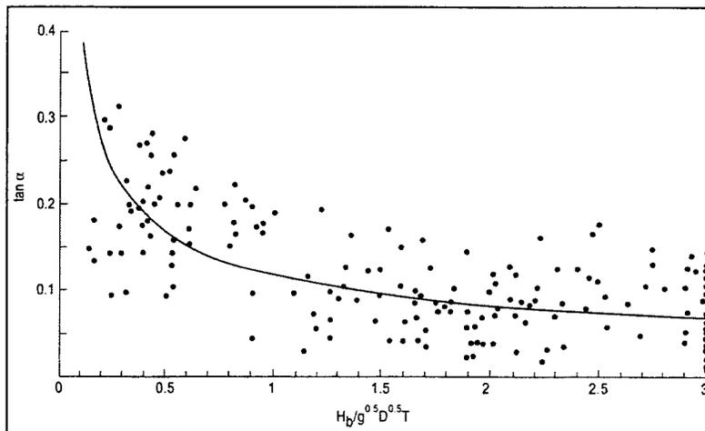
Figure#24 Data points generated when the measured beachface slope is plotted against the dimensionless parameter  $\left(\frac{H_b}{T\sqrt{gD}}\right)$ . The least square fit is also shown. From Short (1999).
