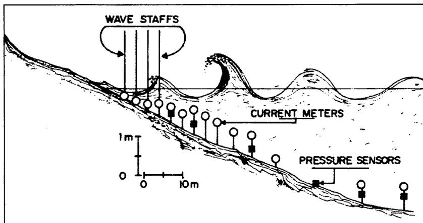
Figure#12 A schematic diagram showing the location of wave and longshore velocity sensors deployed at Leadbetter beach, California between 30<sup>th</sup> January and 23<sup>rd</sup> February 1980. The mean wave period was 14seconds, with the surface elevation of such a wave shown to scale. Taken from Thornton and Guza (1986).
