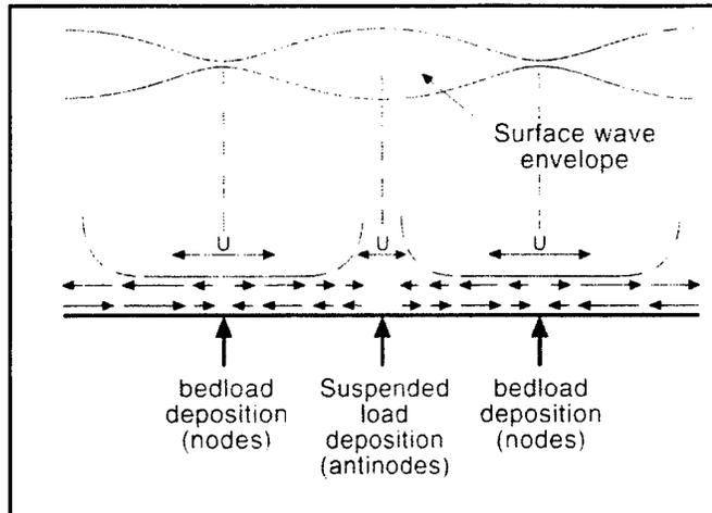
Figure#9 The horizontal velocity ( $u$ ) orbital characteristics beneath a standing infragravity wave and the location of the resulting sand bars when the sediment movement is predominantly in suspended form or in bedload form. Taken from Short (1999).
