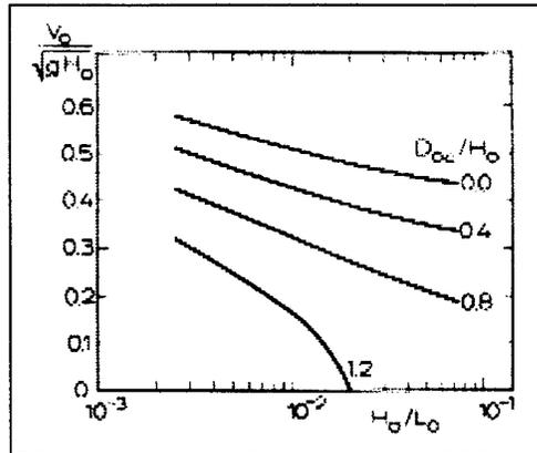
Figure#17 The relationship between the parameter  $\sqrt{g\Delta D_o}$  (defined as  $V_o$ ) as a function of offshore wave steepness ( $H_o/L_o$ ) for differing depths ( $D_{oc}$ ) at the bar crest. Taken from Dalrymple (1978).
