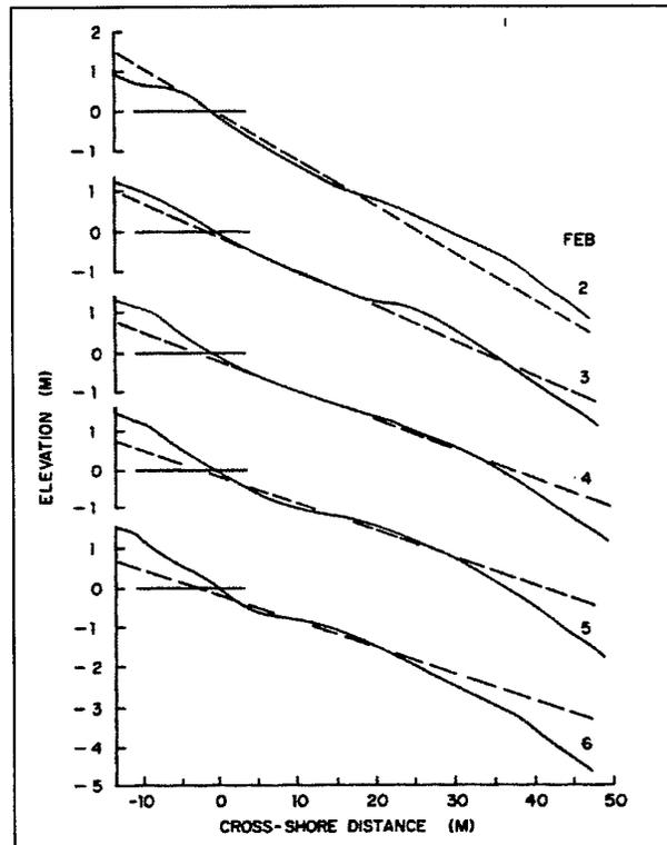
Figure#13 On-offshore beach profiles and mean profiles of Leadbetter beach from the 2<sup>nd</sup> to 6<sup>th</sup> of February 1980. Note how they are all nearly planar (small single bars) with the most planar profile occurring on the 4<sup>th</sup> of February. Taken from Thornton and Guza (1986).
