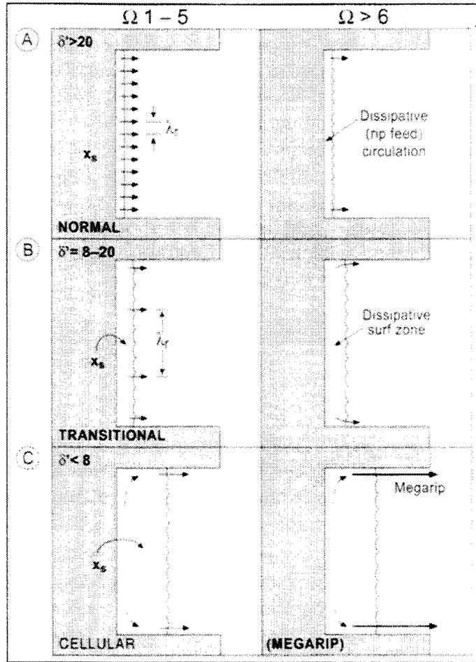
Figure#20 A schematic showing the rip circulation schemes which form as a function of the dimensionless embaymentment parameter and the beach type (depicted by the dimensionless fall velocity ( $\Omega$ )). Taken from Short (1999).
