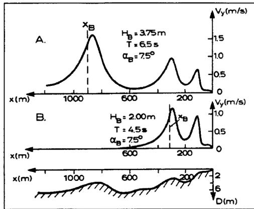
Figure#15 Calculated longshore velocities ( $V_y$ ) for a barred coastal profile for two offshore wave characteristics. Note the location of the maximum velocity over the bar crest although high density data has it located in troughs.  $T$  is the wave period. Taken from Fredsoe and Deigaard (1992).
