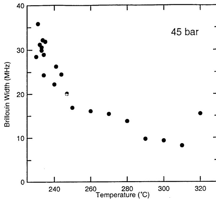
Fig. 7. The peak width observed in stimulated Brillouin scattering for n-hexane at 1064 nm for a pressure of 45 bar as a function of temperature.
