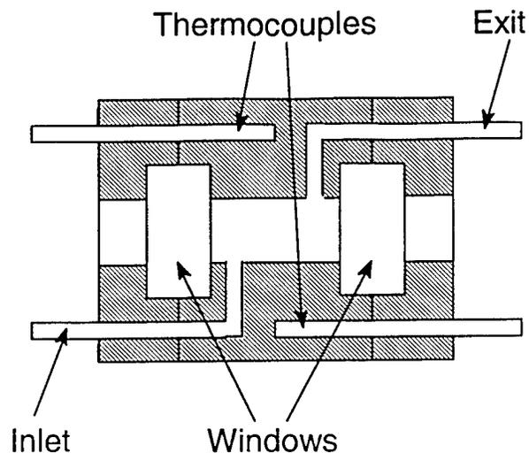
Figure 3. Schematic diagram of the supercritical cell.
