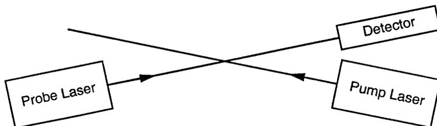
Figure 1. Basic experimental arrangement for stimulated scattering measurements.
