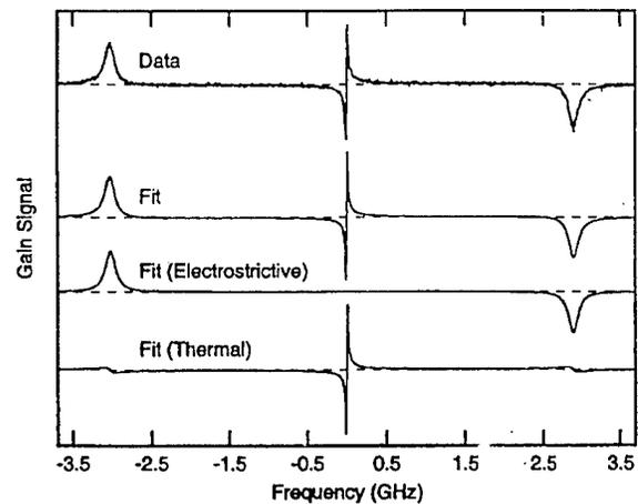
Fig. 2. Stimulated Rayleigh-Brillouin spectrum for *n*-hexane at  $1.064 \mu\text{m}$  (top curve), fits to the data (middle curves), and electrostrictive and thermal components of the fit (bottom curve). The dashed lines indicate the zero gain level for each curve.
