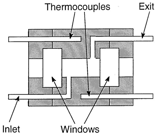
Fig. 2. Schematic diagram of the supercritical cell.
