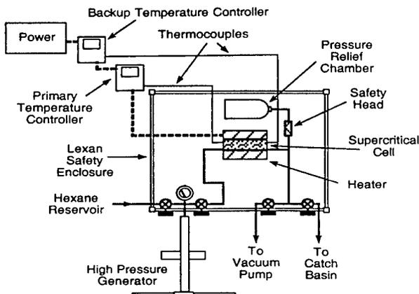
Fig. 3. Overall high pressure system.
