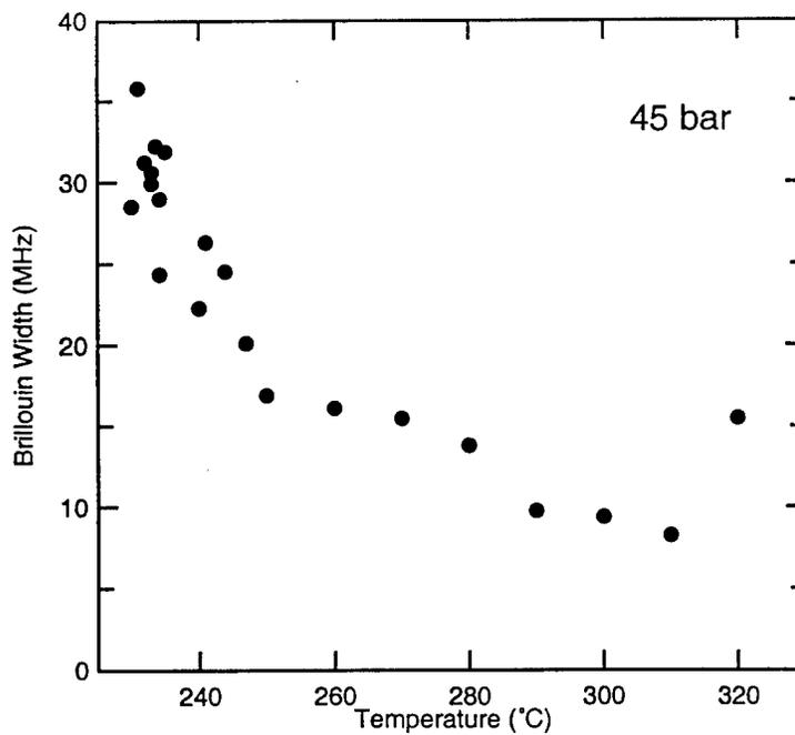
Figure 12. The peak width observed in stimulated Brillouin scattering for n-hexane at 1064 nm for a pressure of 45 bar as a function of temperature.
