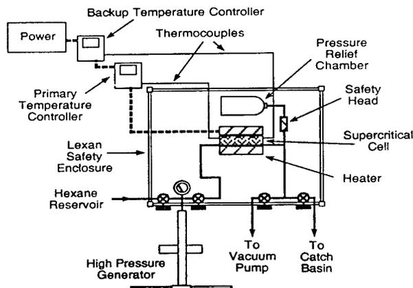
Figure 4. Overall high pressure system.
