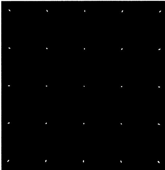
Figure 4. Diffraction image of a fiber optic light source (632.8 nm)
