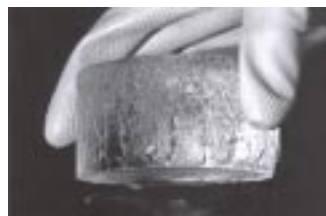
c. Side view of Sample B with its top downward. Note candled ice grains and possible surface melting at lower right.
