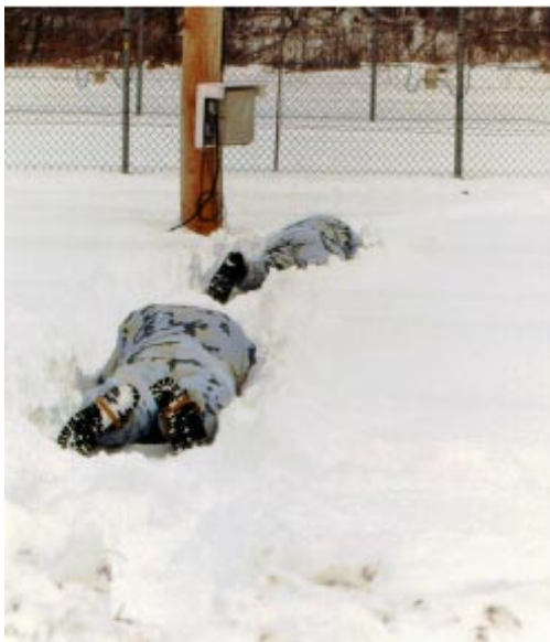
Figure 15. Two intruders crawling through PIR's detection zone. Second intruder uses trench created by first intruder's passage through the 19-cm-deep snow.
