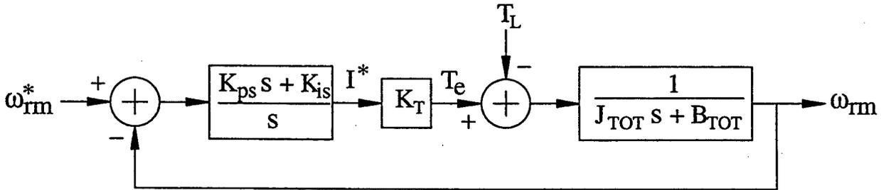
Figure 7. Closed-loop speed control system
