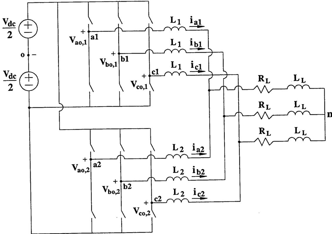
Figure 4. Two paralleled inverters powering an R-L load
