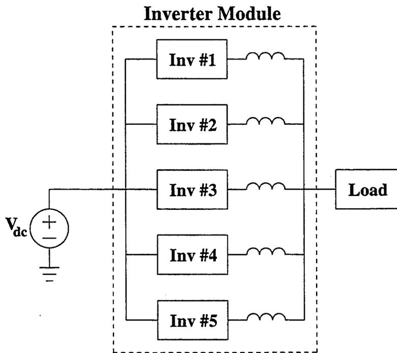
Figure 1. Inverter module containing five inverter submodules
