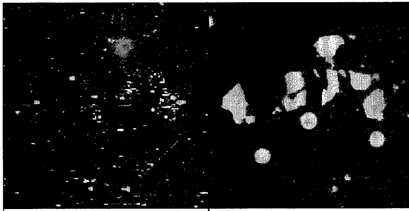
Figure 1. AFM image of intermetallic particles in AA2024-T3. Both images 80 x 80 \mu\text{m} , Left, topographical map with 100 nm z scale, right, Volta potential map with 1.5 V z scale [1].
