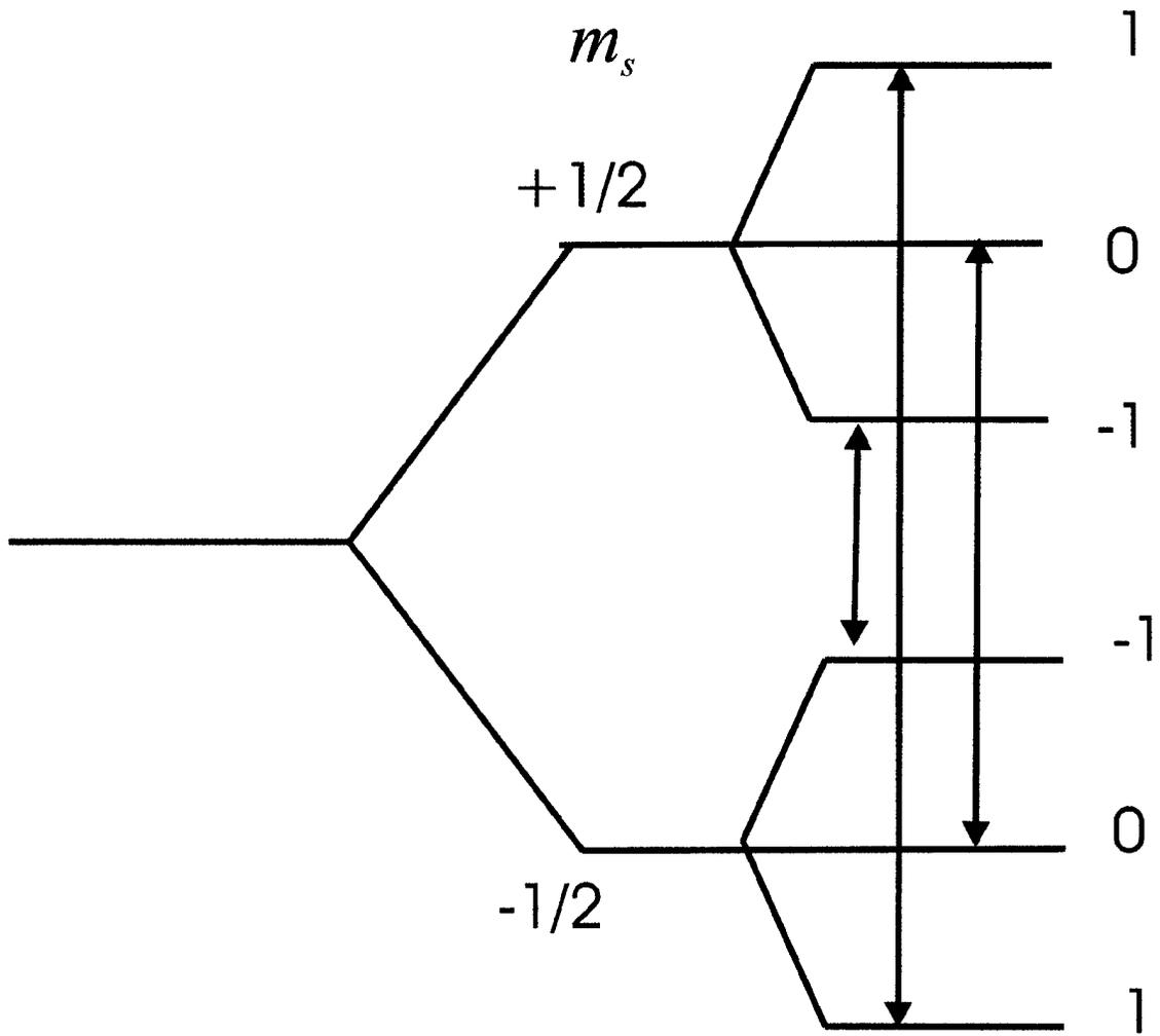
Figure 2.1-3 Energy levels with splitting caused by hyperfine coupling with nuclear spin of  $I=1$ . Arrows indicate allowed transitions.
