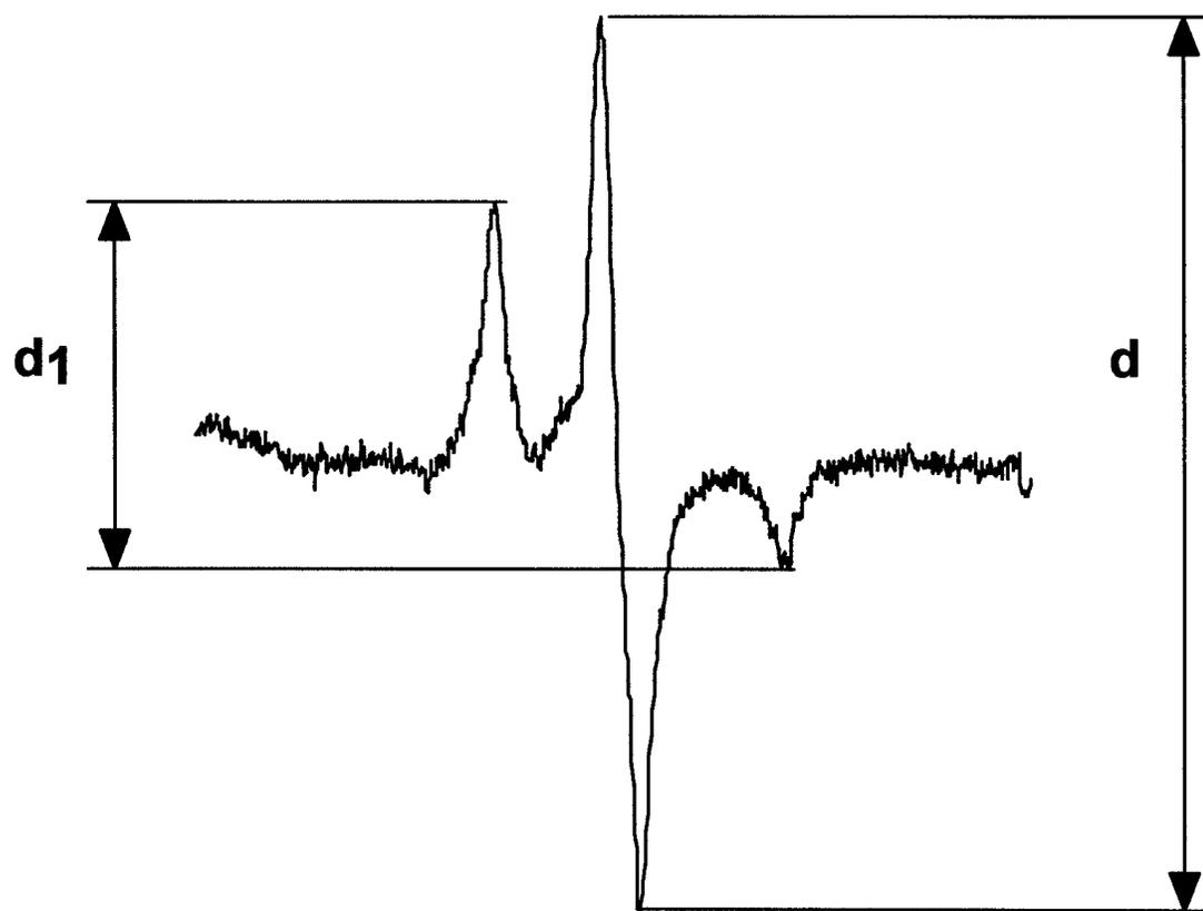
Figure 2.2-1 Low temperature EPR spectrum showing measurements  $d$  and  $d_1$ . If the ratio  $d_1/d$  is  $>0.4$  it is an indication there is a dipolar interaction between two spins in close (within 24 Å) proximity
