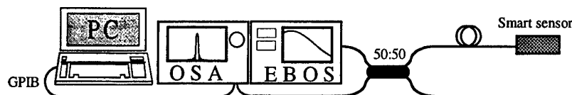
Fig. 4 Experimental set-up used for monitoring smart sensor plates.
