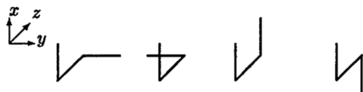
Figure 1: Basic wire structures. Two chiral cranks of opposite handedness (enantiomorphs), a non-chiral staple and a non-chiral crank.
