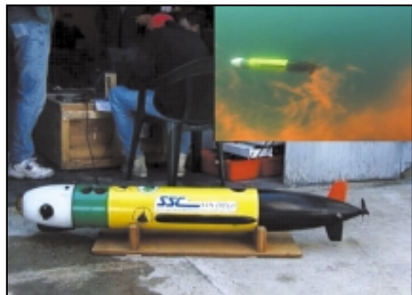
FIGURE 3 AUV (REMUS) used in plume-mapping experiments. Sensing elements are contained in the white nose cone, a current profiler is in the green section, and vehicle controls and batteries are in the central yellow section. The inset shows the AUV while deployed in a plume mapping experiment. [Images courtesy of SPAWAR.]
