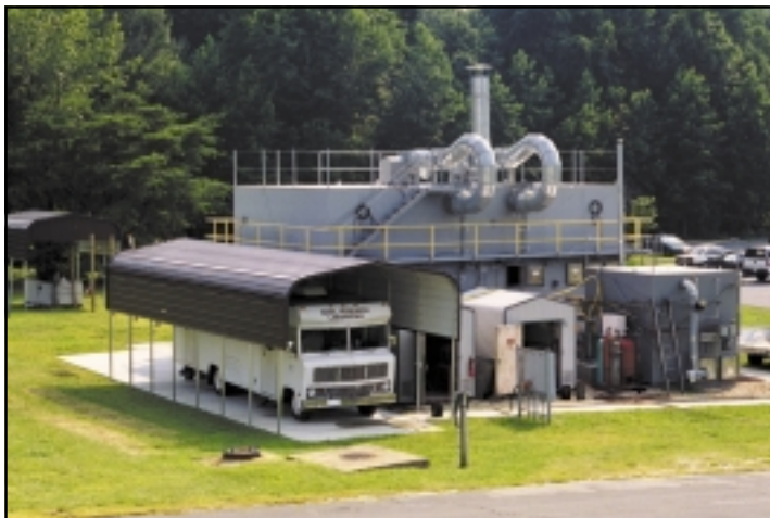
FIGURE 13 Fire test facility at the NRL Chesapeake Bay Detachment. The two enclosures at the rear (285 cubic meters) and the right (27 cubic meters) of the picture are used for testing different sized shipboard compartments.
