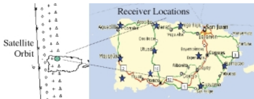
FIGURE 1 Geometry for the ionospheric tomography experiment in Puerto Rico.
