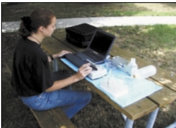
FIGURE 2 Setup for field operation of current-generation NRL flow biosensor. To assay for explosives and measure concentrations, samples are injected into the instrument and moved by a fluid stream to immobilized antibodies. Any increase in fluorescence is observed within minutes and stored on the computer for later data analysis.
