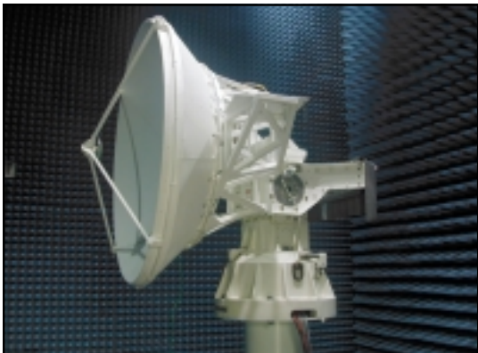
FIGURE 2 WARLOC radar antenna.
