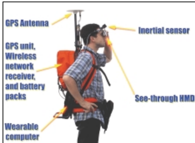
FIGURE 6 Current BARS development system. This system is developed using COTS products, hence its size. (This system might be a familiar sight to regular users of the Building 28 cafeteria.)
