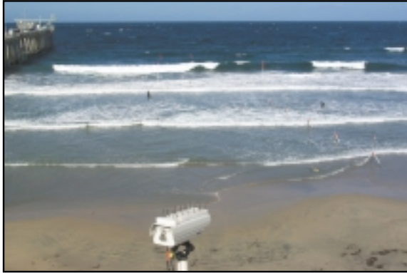
FIGURE 12 Field set up for typical current meter deployment. The instrumentation can be seen as the tripods extending offshore from the right. The camera located in lower center of image is used for PIV.
