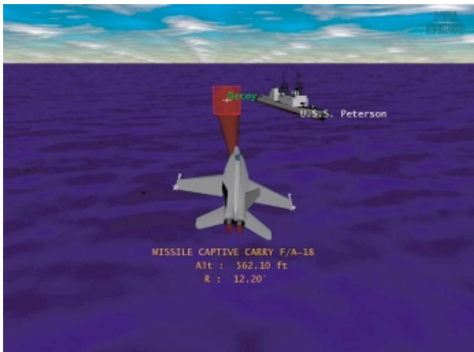
FIGURE 10 SIMDIS display of F/A-18 captive carry missile seeker track.
