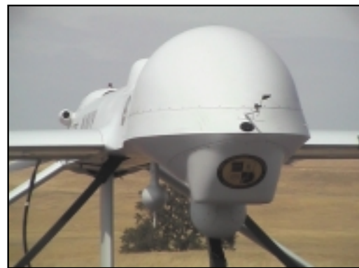
FIGURE 4 WAR HORSE hyperspectral target detection system installed aboard the NPS Predator UAV.
