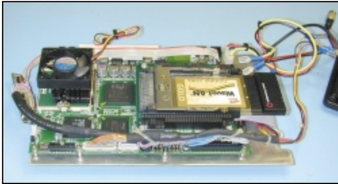
FIGURE 8 Wearable computer complete with IEEE 802.11 RF local area network.
