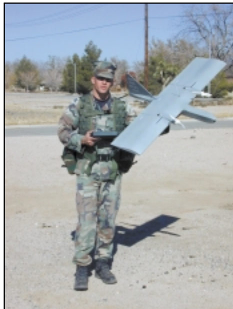
FIGURE 10 A U.S. Marine wearing the ground control station while holding the Dragon Eye UAV.
