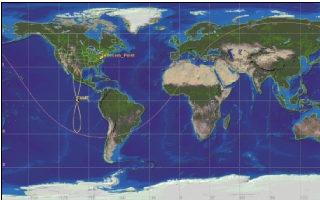
FIGURE 3 Graphical representation of nominal FAME ground track, tracking station, and tracking station field of view.
