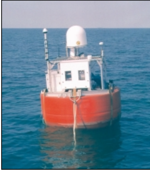
NRL's satellite-linked buoy system during a recent ocean deployment. Data from one or two arrays of hydrophones are collected and stored within the buoy, and simultaneously transmitted to ships in the vicinity and to shore using RF and satellite communications.
