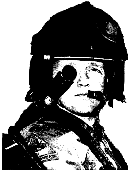
Figure 2. The AH-64 Integrated Helmet and Display Sighting System (IHADSS).
