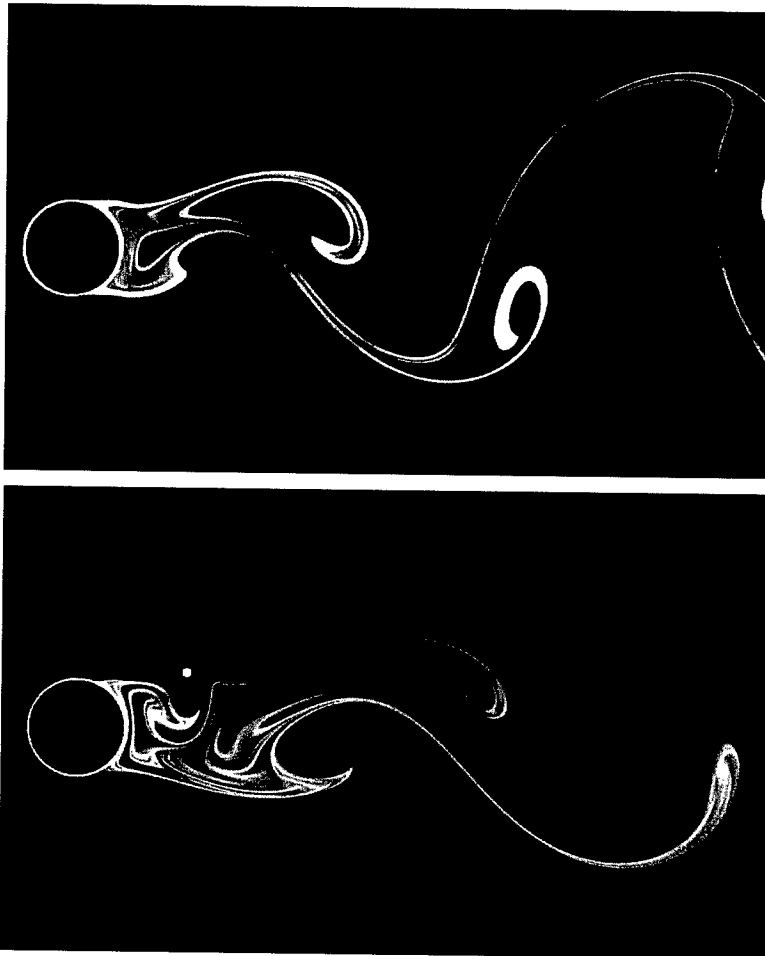
Figure 5. Flow visualization comparison at Re = 100 , \alpha = 30^\circ , and R/D = 1.4 .
