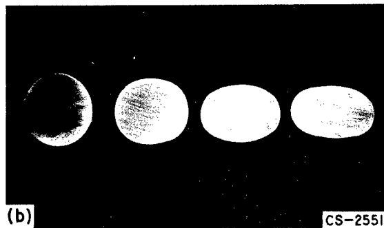
FIGURE 71-10.—Deformation of cold-forged bars of strongest tantalum-modified alloy.
