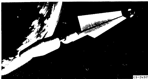
FIGURE 46-6.—Manned, electrically propelled, interplanetary spacecraft. Estimated power requirement, 10 to 30 megawatts.
