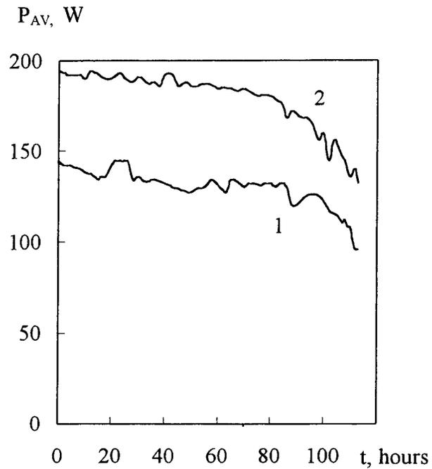
Fig.5. Dependencies of the average radiation power in stationary mode versus the operating time of TEA-CO<sub>2</sub> lasers with  $V_{a1}=28*2*0.6 \text{ cm}^3$  (1) and  $V_{a2}=45*2.5*0.8 \text{ cm}^3$  (2).
