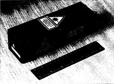
Fig. 6. Electrooptical Q-switch diode-pumped laser head
