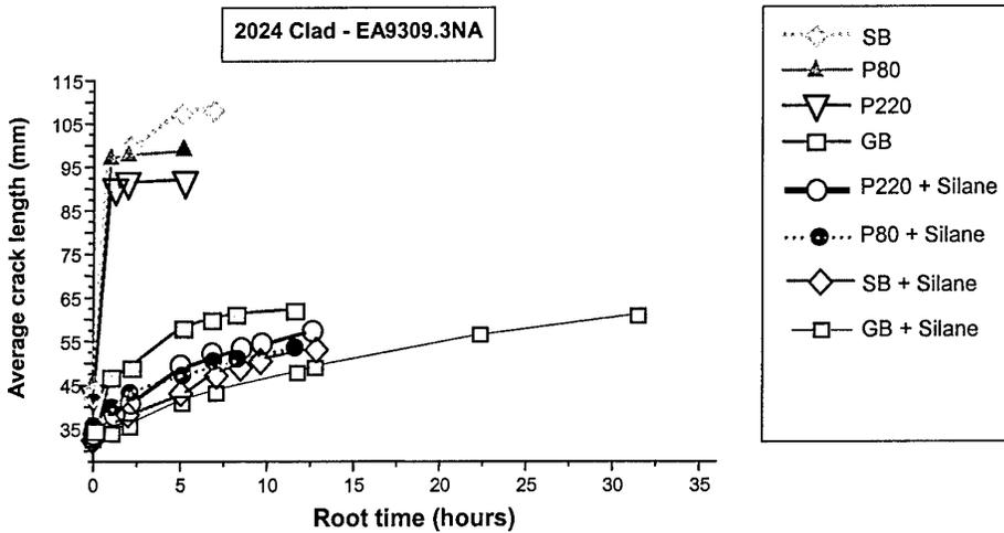
Figure 1 Bond durability data for Al-2024 T3 clad aluminium bonded to EA9309.3NA paste adhesive as a function of the surface pre-treatment.
