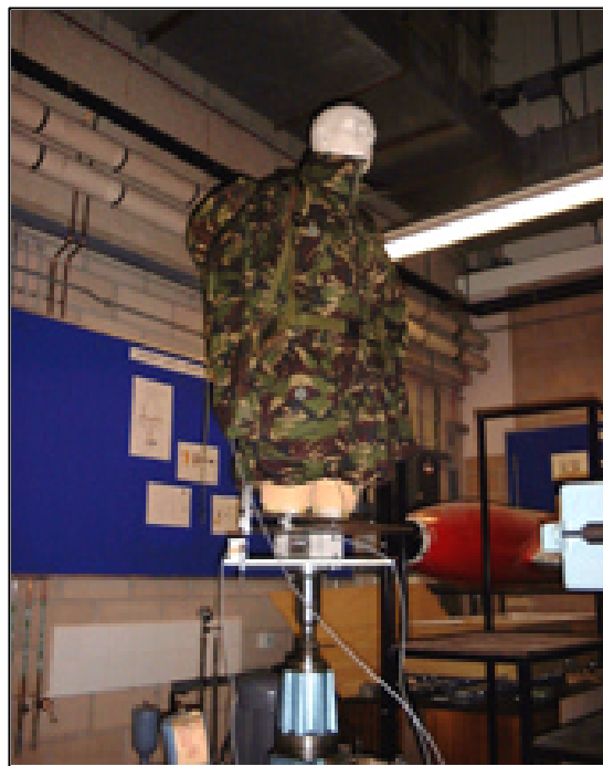
Figure 3. Photo of Load Carriage Rig
