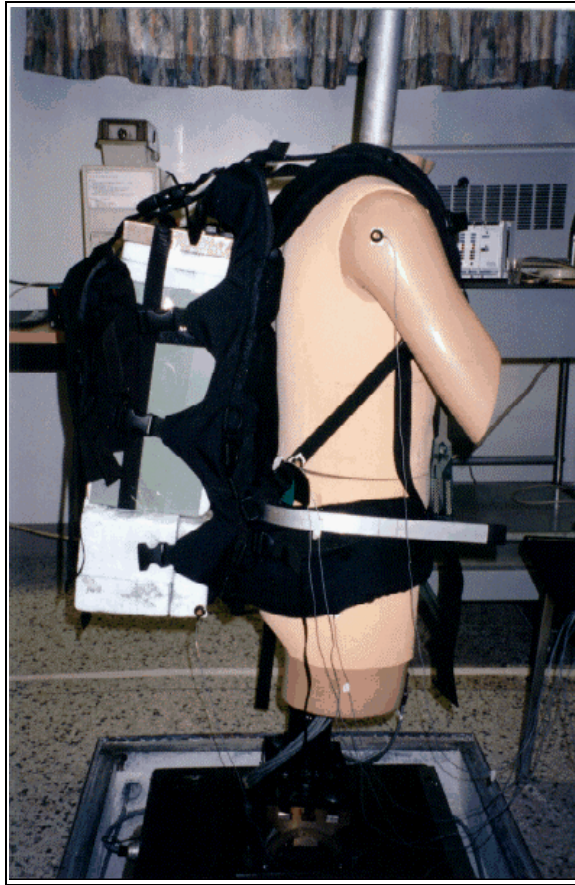
Figure 1. Experimental Setup (41 degree shoulder strap angle).
