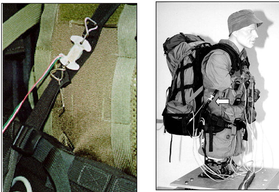
Figure 4. Custom strap force transducers for measuring strap tension.
