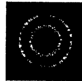
FIG. 2. Typical far field intensity pattern for the signal during the transient behavior as it results from numerical simulations.
