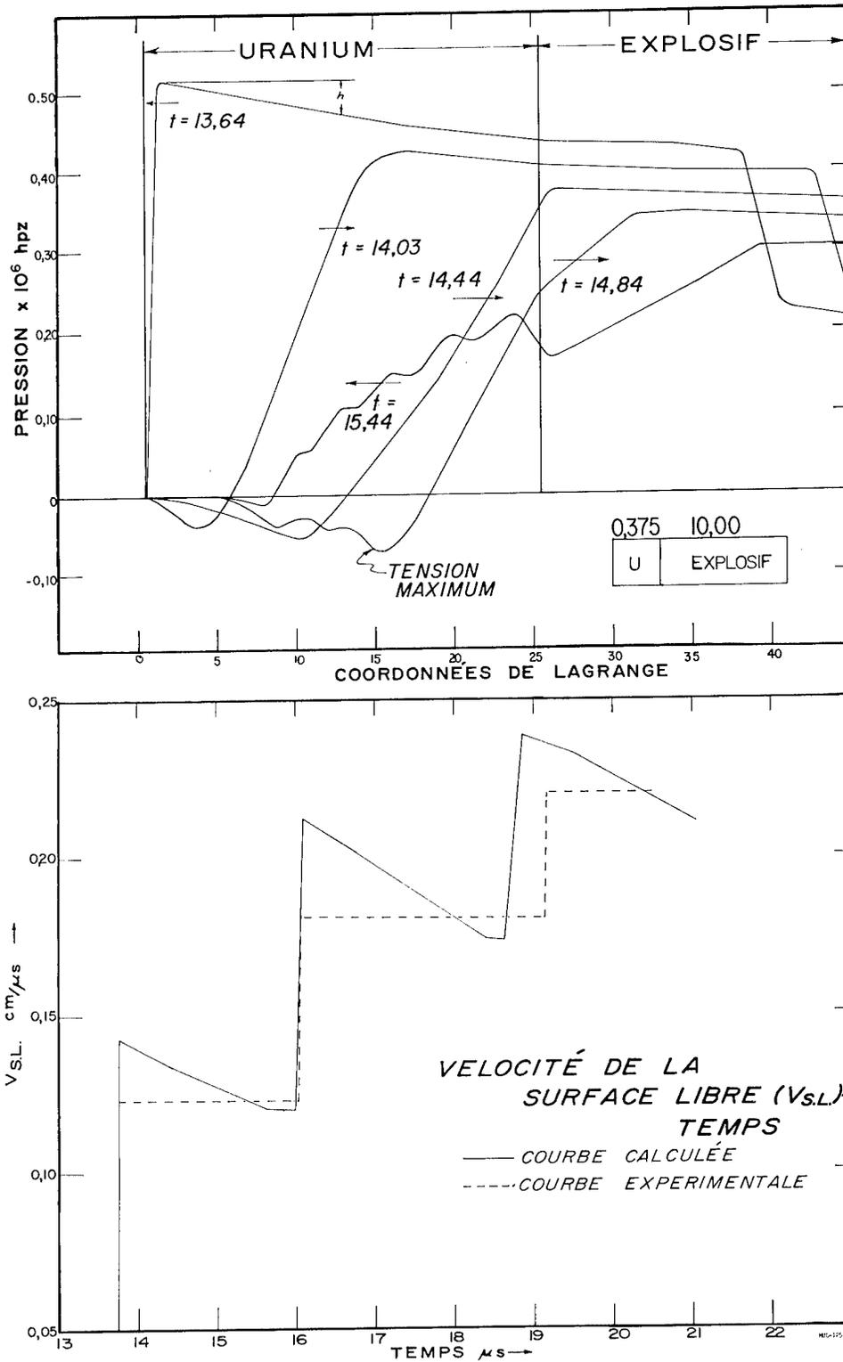
Fig. 1. Top: Pressure profiles at different times (pressure - Mb, time - μsec). Bottom: Front surface velocity vs time.
