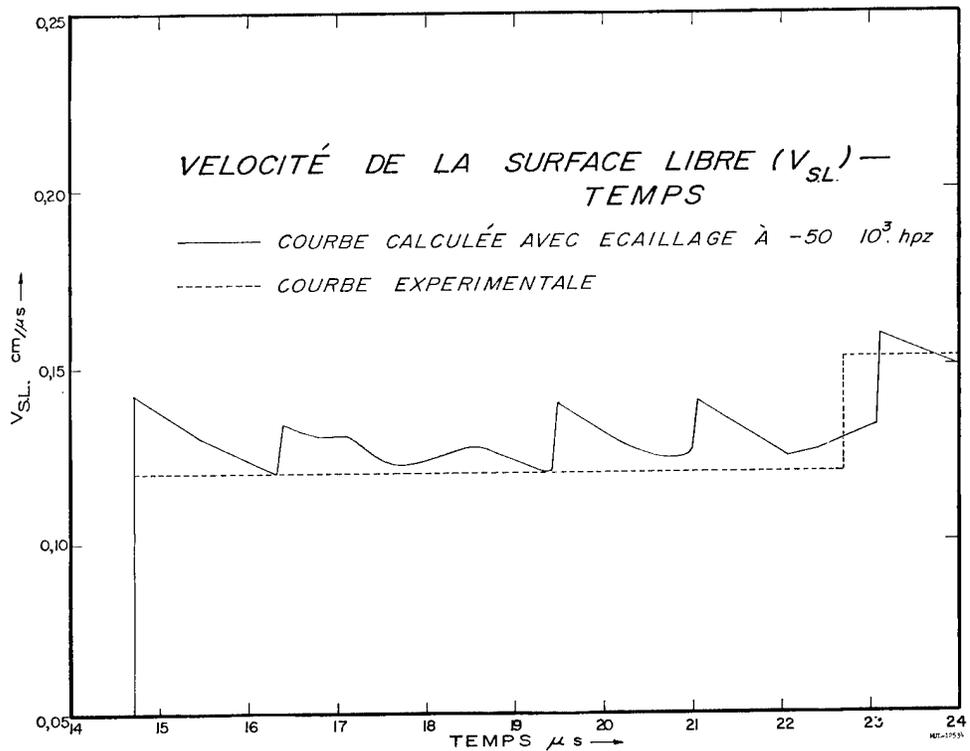
Fig. 5. Top: Distance vs time of uranium ("ecaillage" = spall). Bottom: Uranium front surface velocity vs time (where spall was allowed to occur at - 50 kb).
