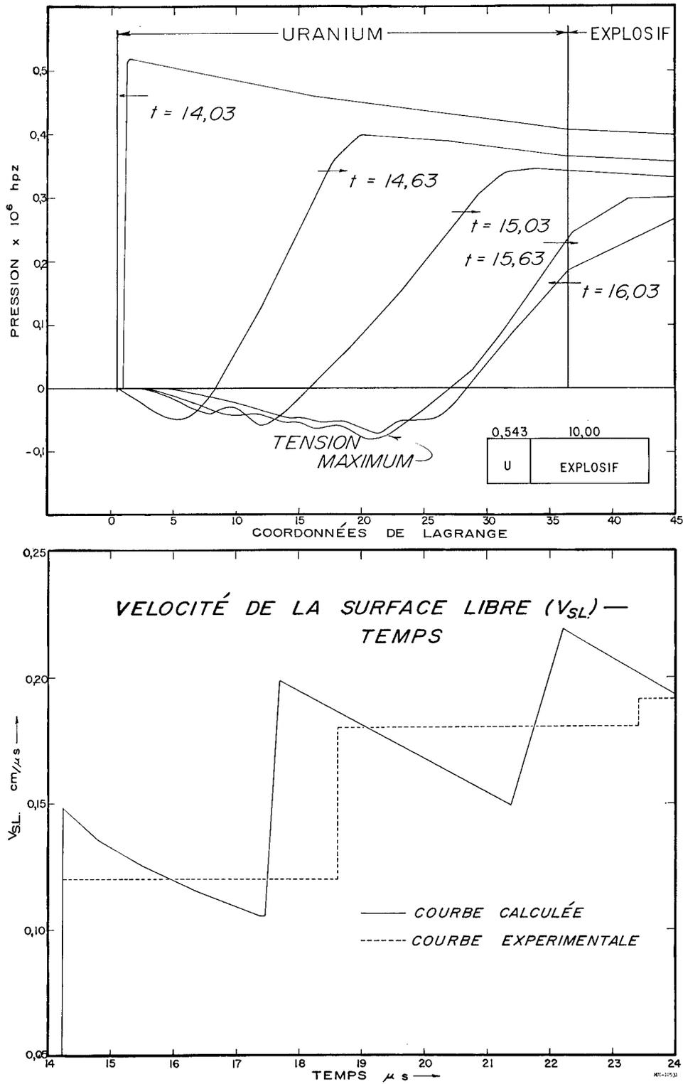
Fig. 2. Top: Pressure profiles at different times (pressure - Mb, time μsec). Bottom: Front surface velocity vs time.
