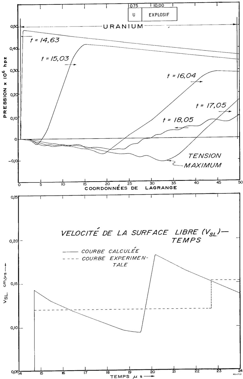
Fig. 3. Top: Pressure profiles at different times (pressure - Mb, time - μsec). Bottom: Front surface velocity vs time.
