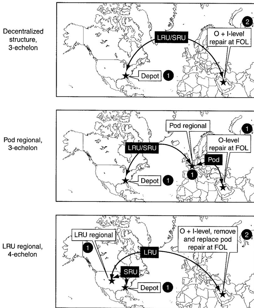
Figure 3.3—LRU Repair Consolidation Adds Another Echelon
