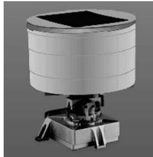
Remote sensing: star tracker camera used on Clementine spacecraft that mapped the moon's surface
