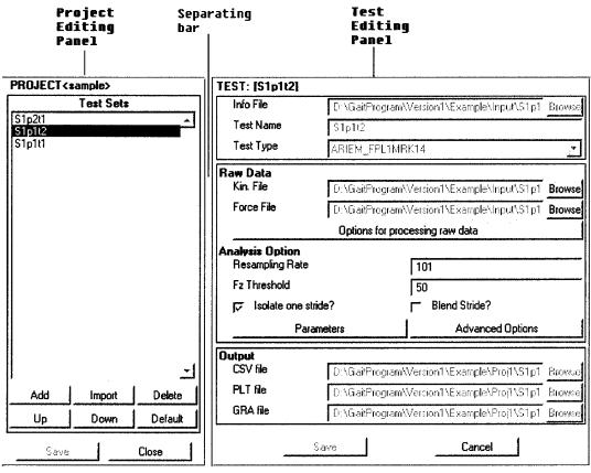
**Project Editing Panel** contains a listbox listing all tests in the project; an **Add** button to add a test to the project; an **Import** button to import a test into the project; a **Delete** button to remove a test from the project; an **Up** and a **Down** button to change the sequence of tests in the project; and a **Default** button to change the default test setting. It also contains a **Save** and a **Close** button to save the changes to the project and to close the project.
