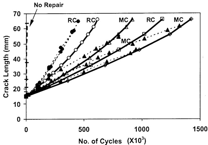
Figure 1. Experimental and numerical results for fatigue crack growth (For recommended cure cycle (RC), experiment : --●--, prediction with strain rate effect : —○—, prediction with linear elasticity : —□—. For modified cycle (MC), experiment : --▲--, prediction with strain rate effect : —△—, prediction with linear elasticity : —◇—.)
