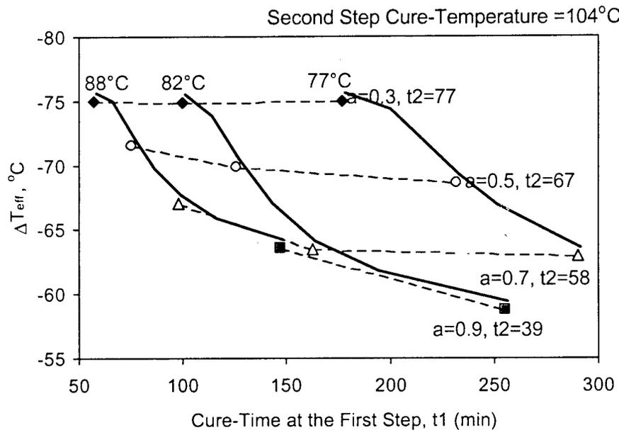
Figure 3.  $\Delta T_{eff}$ 's for two-step cure cycles with 104°C second step cure-temperature ( $a$  : degree of cure after the first step cure,  $t_1$  (min) : the cure-time taken at the first step cure,  $t_2$  (min) : the minimum required cure-time at the second step with 104°C corresponding to the degree of cure after the first step cure, the temperatures of 88°C, 82°C, and 77°C indicate the cure-temperatures at the first step)
