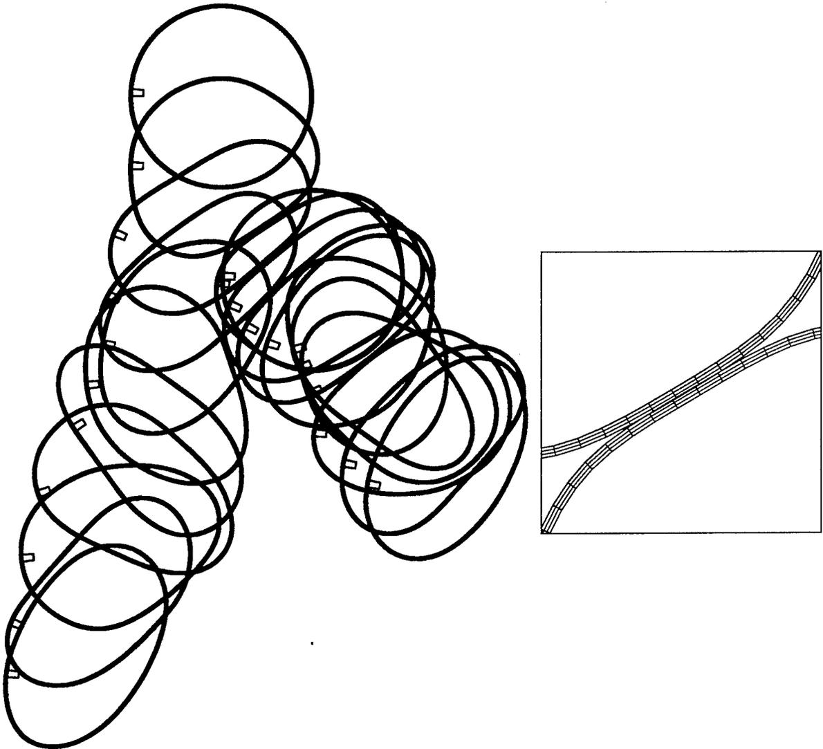
Figure 5: Two ring impact problem, dynamic configurations,  $t = [0, 2, 4, \dots, 20]$ . The inset shows a zoom of the contact interface at a typical time step. The velocity update algorithm is seen to produce stable results and to facilitate accurate constraint enforcement.
