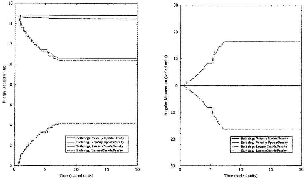
Figure 6: Two ring impact problem: (a) energy evolution, (b) angular momentum evolution.
