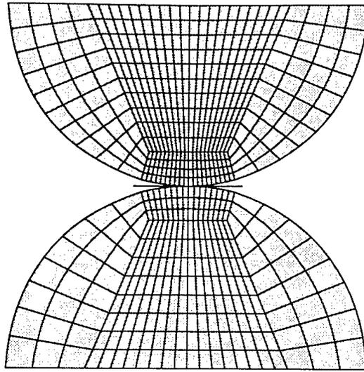
Figure 9: Discretization, cylinder on cylinder contact problem.
