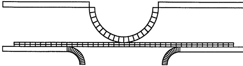
Figure 11: Undeformed configuration of the sheet-drawbead system.
