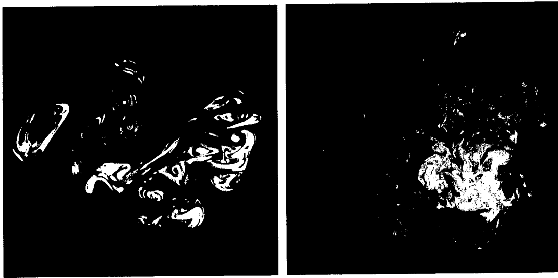
FIG. 10 Jet-fluid concentration in a transverse slice of jet at downstream location x/d_j = 50 for V_r \simeq 10.1 . Left: Re_j = 1.0 \times 10^3 . Right: Re_j = 10 \times 10^3
