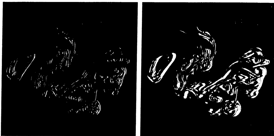
FIG. 13 Two-dimensional scalar-difference field. Left: Horizontal increment of 2 pixels. Right: Horizontal increment of 16 pixels.
