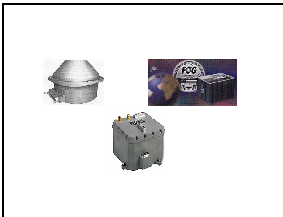
Figure 8. Sampling of New or Proposed Tactical Grade INS Systems
