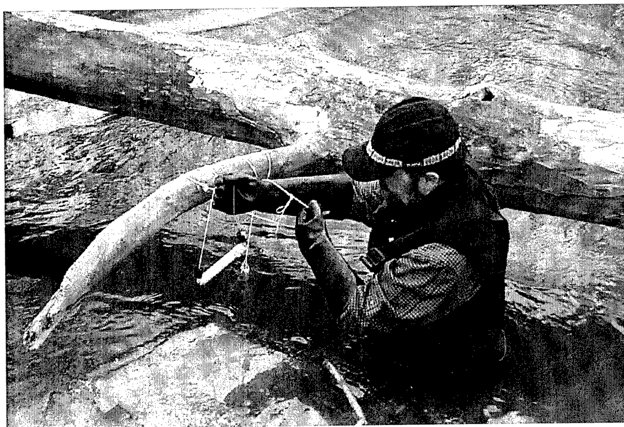
Figure 4. Flow-through microbial sampler about to be suspended in open water upstream from the water quality sensors. Note sheet ice growth in river; frazil ice was also present in deposits beneath the sheet ice
