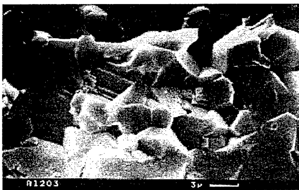
Fig.1 SEM of fracture surface of aluminas hot-pressed at high temperatures (1600-1720°C).
