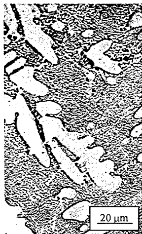
Pic. Microstructure of the eutectic alloy of the Al-Ge-Mg ternary system.
